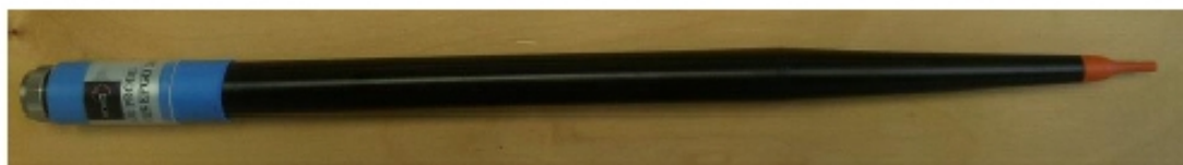
Figure 1 – MVG COMOSAR Dosimetric E field Dipole
