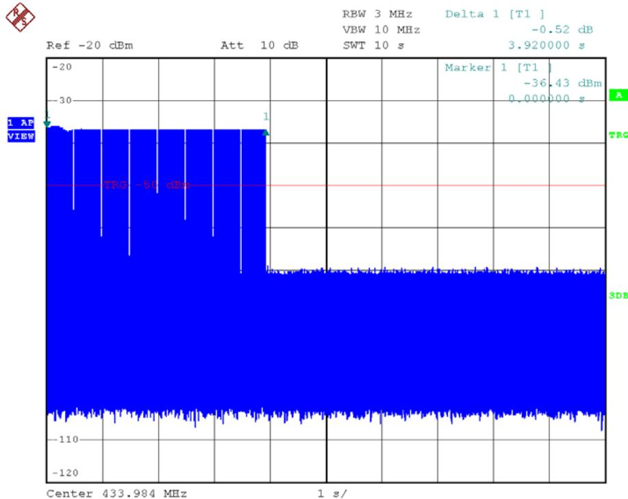
Timing – Pursuant to FCC Part 15 Section 15. 231 Requirement
