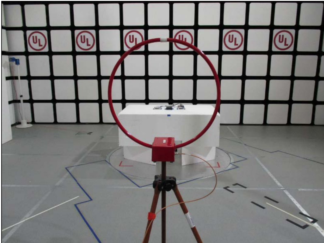
Radiated Emissions 9kHz – 30MHz
