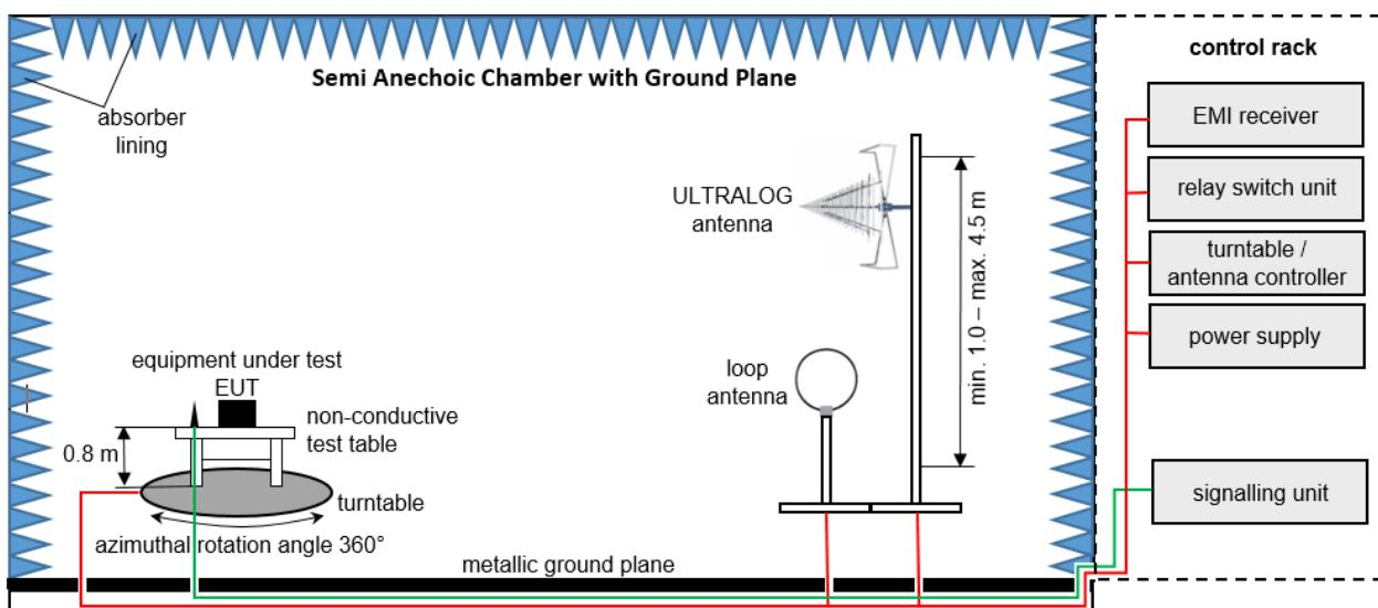
Measurement distance: ULTRALOG antenna 3 m; loop antenna 3 m
