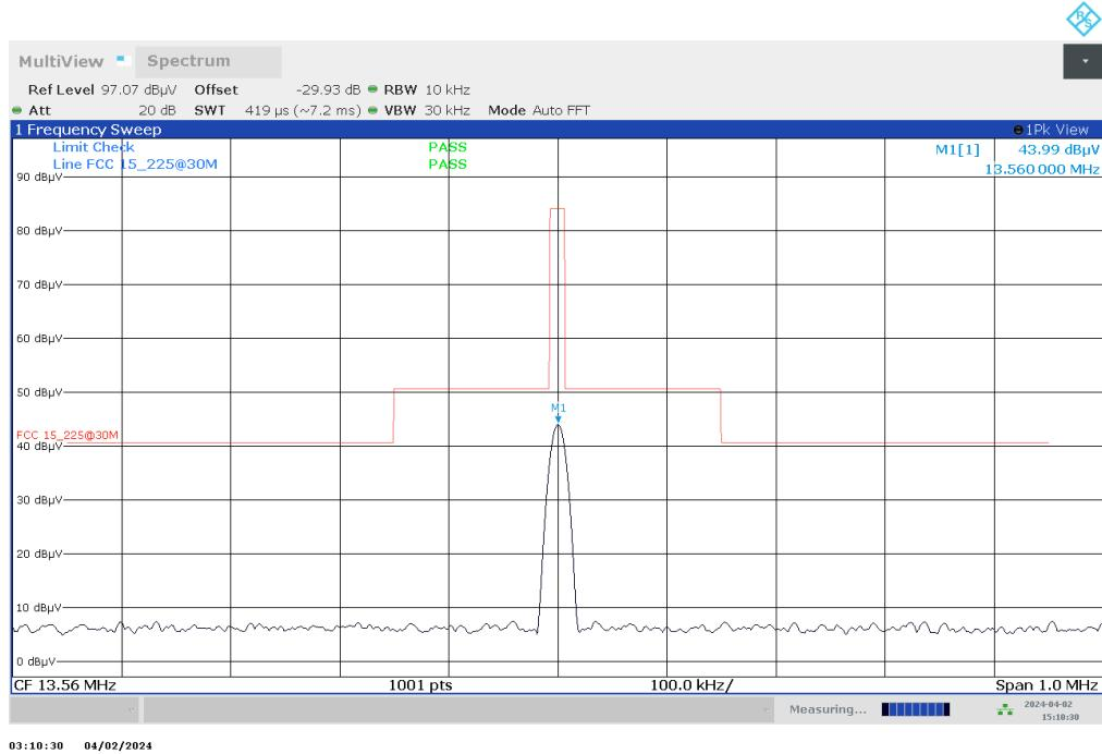
Plot no. 7: Frequency tolerance @ +20 °C, EUT A, V<sub>min</sub>
