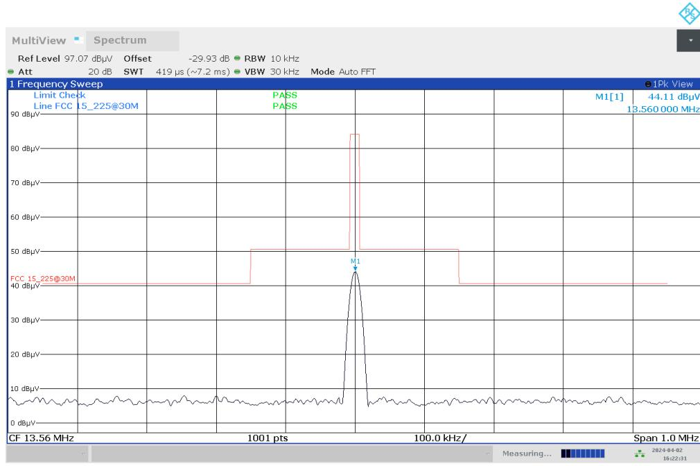
Plot no. 10: Frequency tolerance @ -40 °C, EUT A, Vmin
