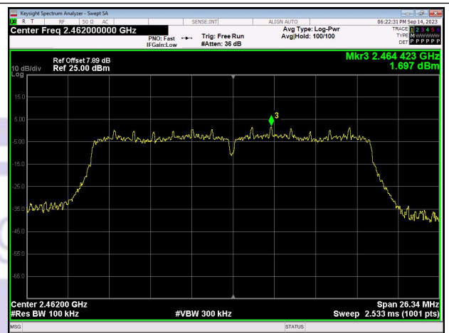
In-Band Reference Level IEEE 802.11n_Channel 11_20MHz_Antenna 0
