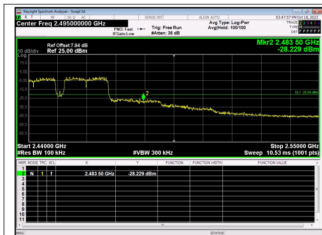
Out Of Band Emission IEEE 802.11n_Channel 9_40MHz_Antenna 0
