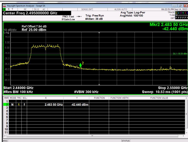
Out Of Band Emission IEEE 802.11n_Channel 11_20MHz_Antenna 0
