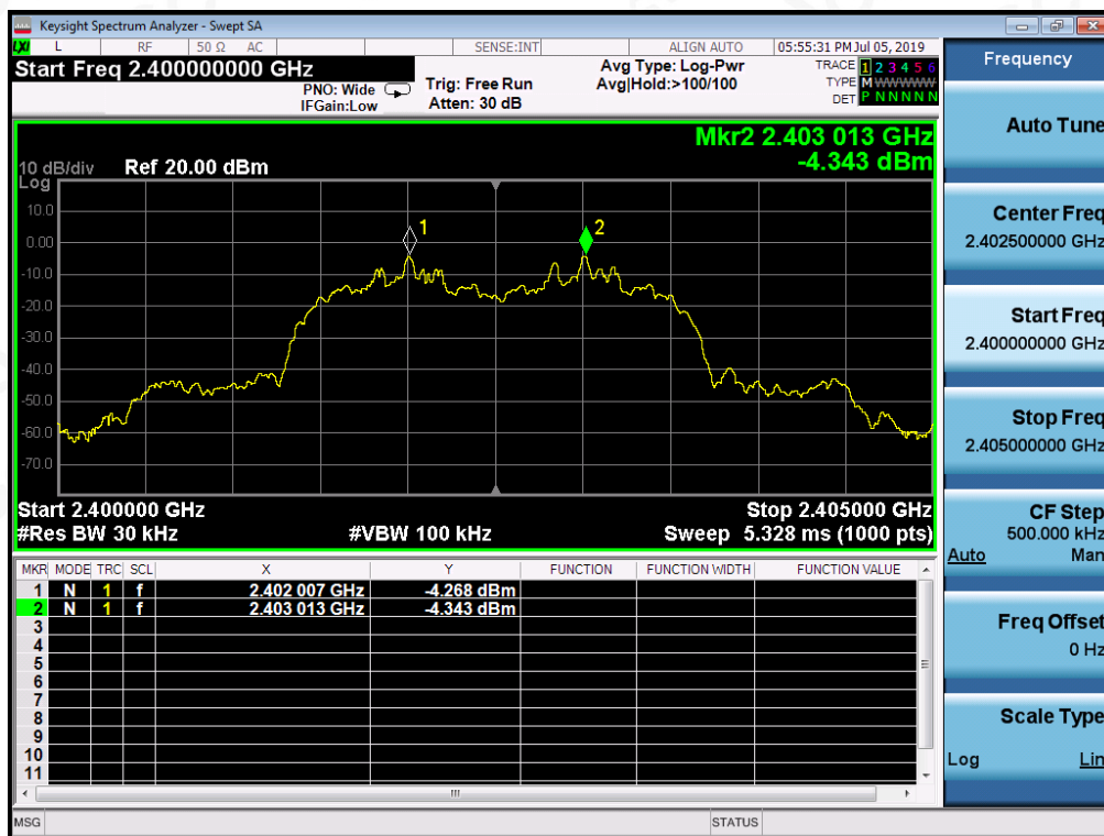
TEST PLOT FOR FREQUENCY SEPARATION
