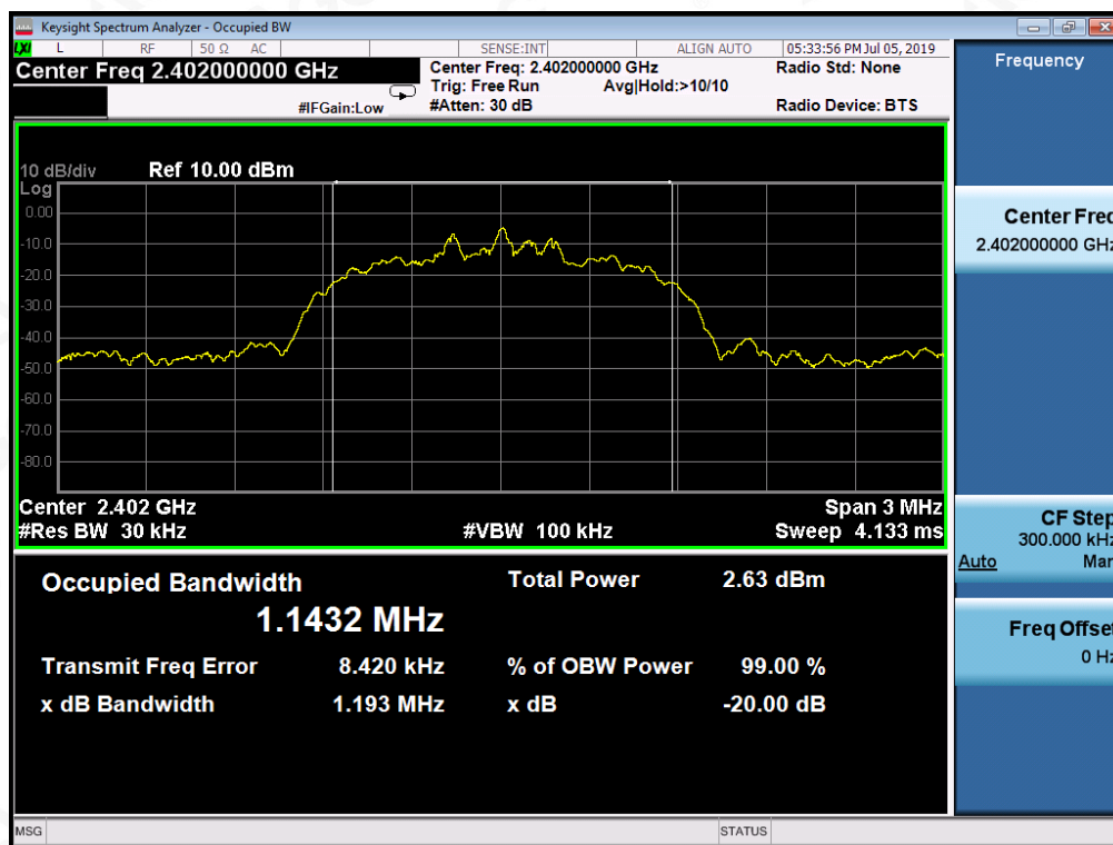
TEST PLOT OF BANDWIDTH FOR LOW CHANNEL
