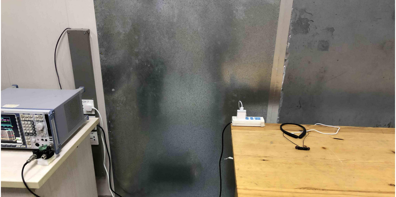
Radiated Spurious Emissions Test Frequency From 30MHz-1000MHz
