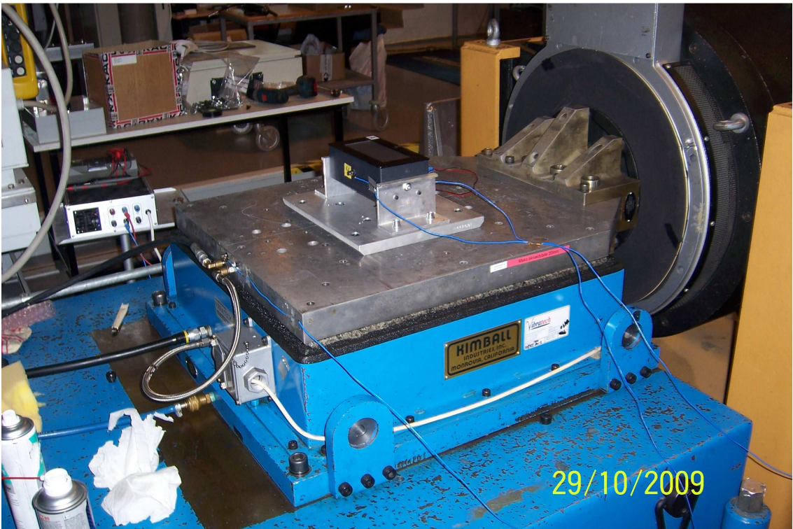
Notes: Test set-up for Vibration in Z axis
