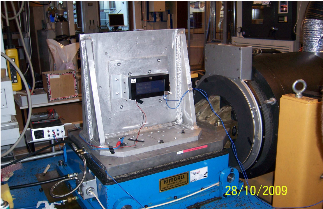
Notes: Test set-up for Vibration in Y axis
