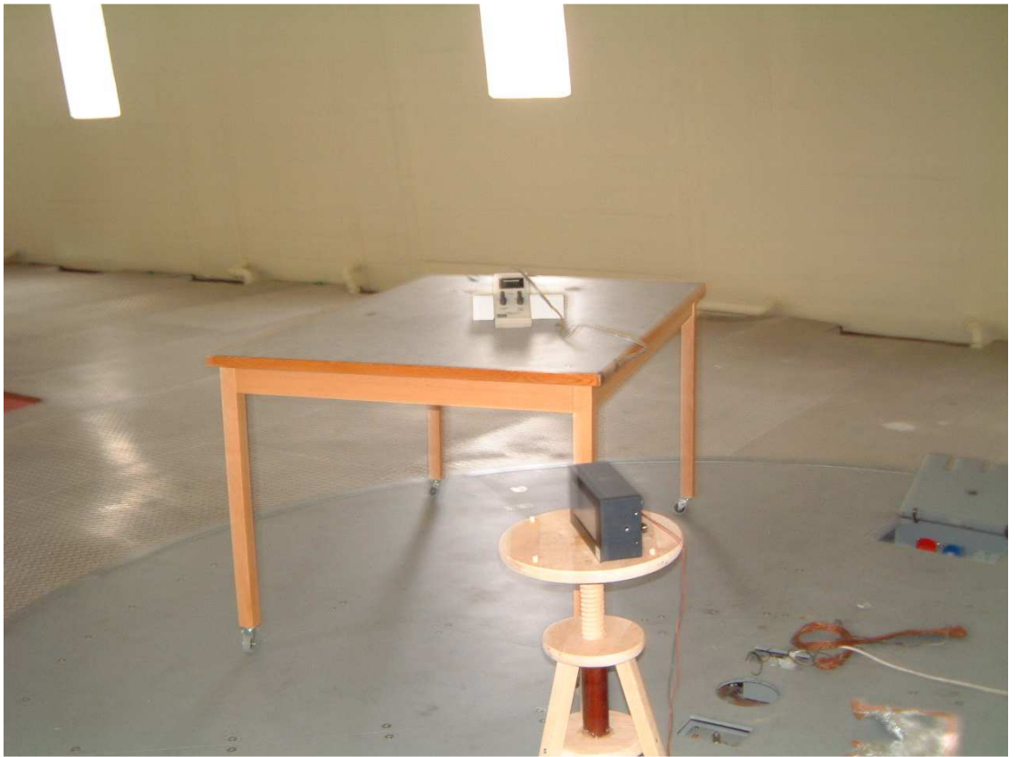
Notes: Test set-up for Compass Safe Distance
