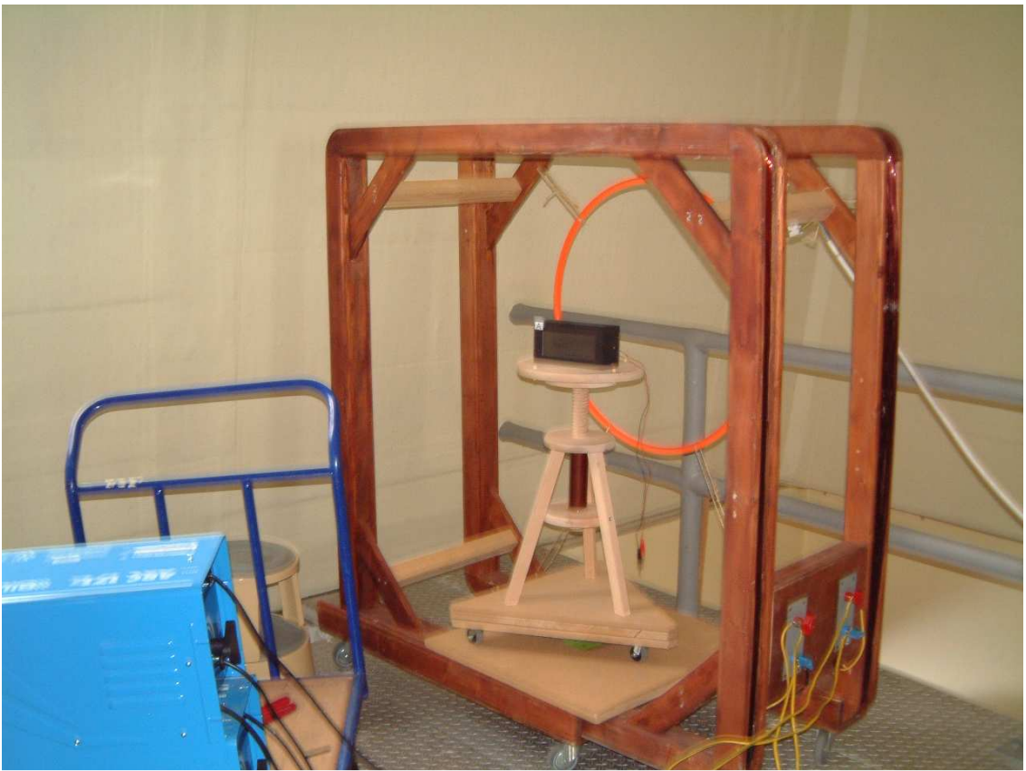
Notes: Test set-up for Compass Safe Distance
