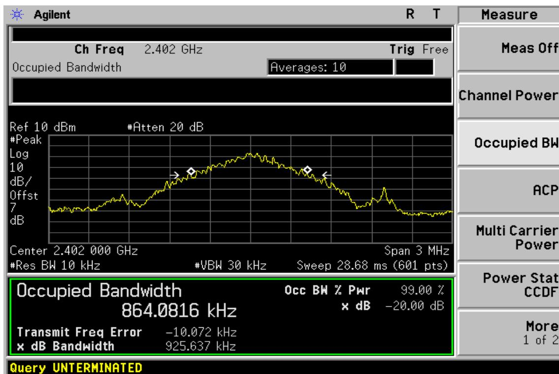
**20dB Bandwidth & 99% Bandwidth Test Data CH-Mid**
