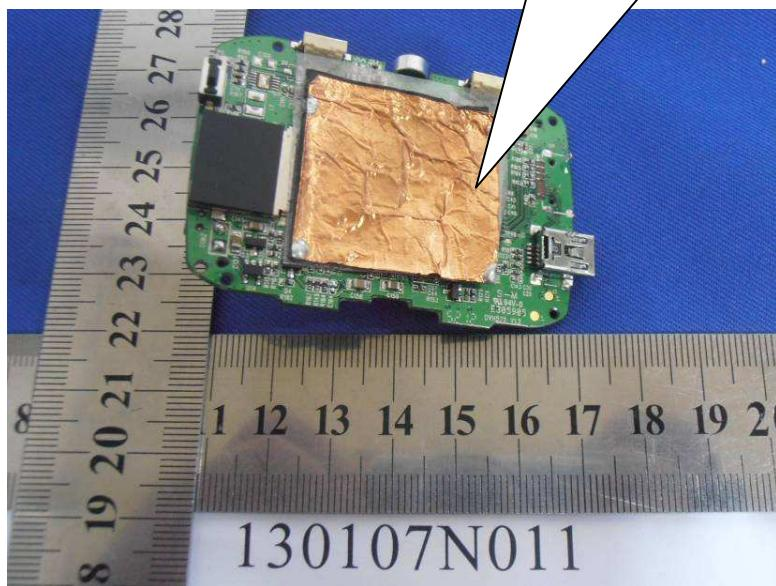
PCB board should add a piece of copper grounding
