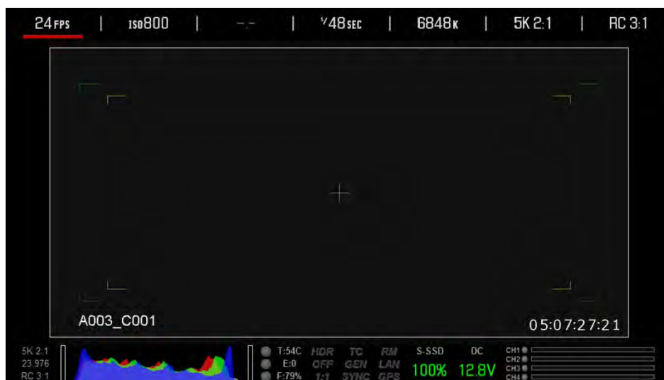
Figure 2: Example of Video Monitor Output – WITHOUT LCD or EVF Connected
