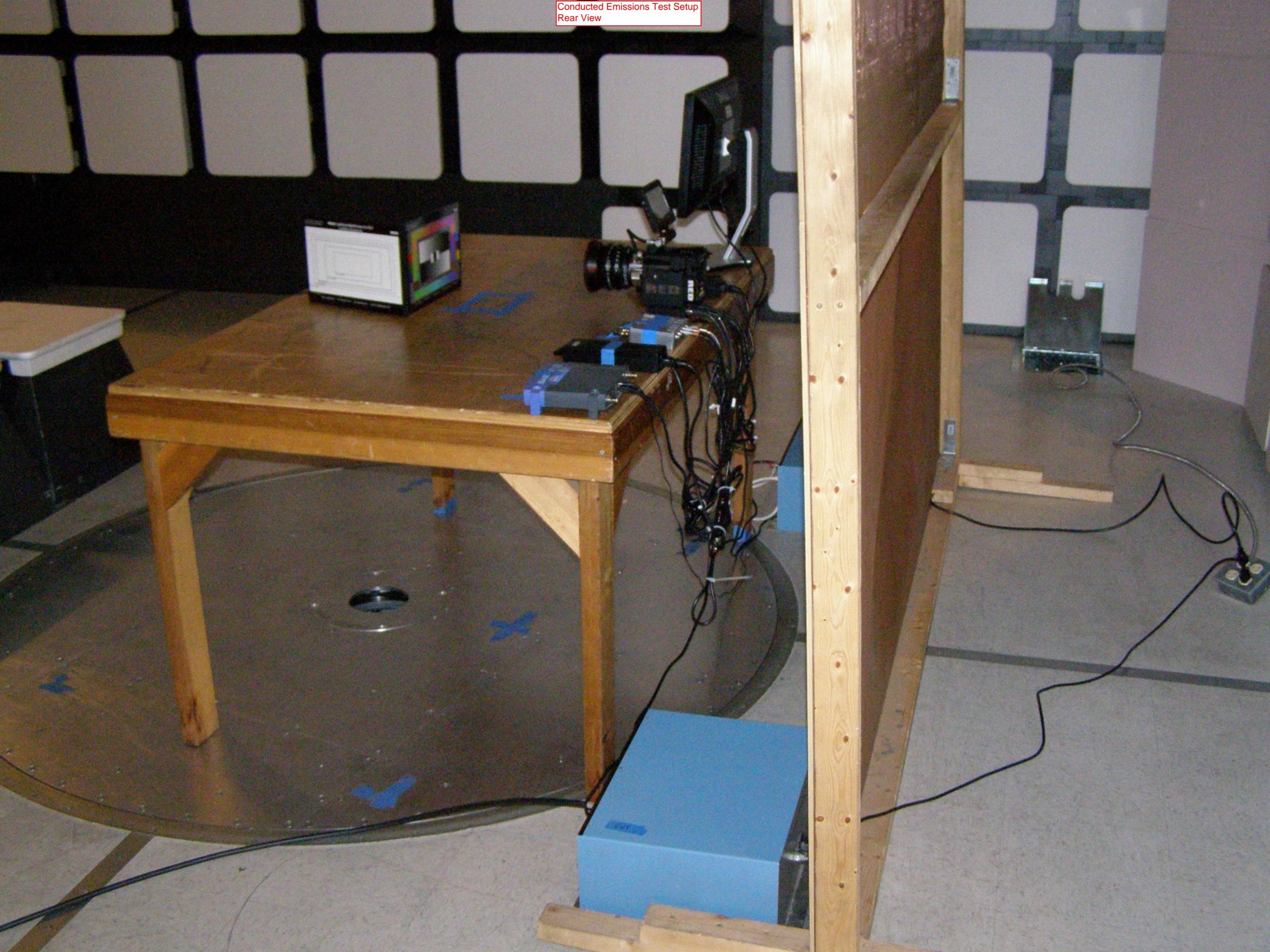
Radiated Emissions Test Setup Below 1GHz
