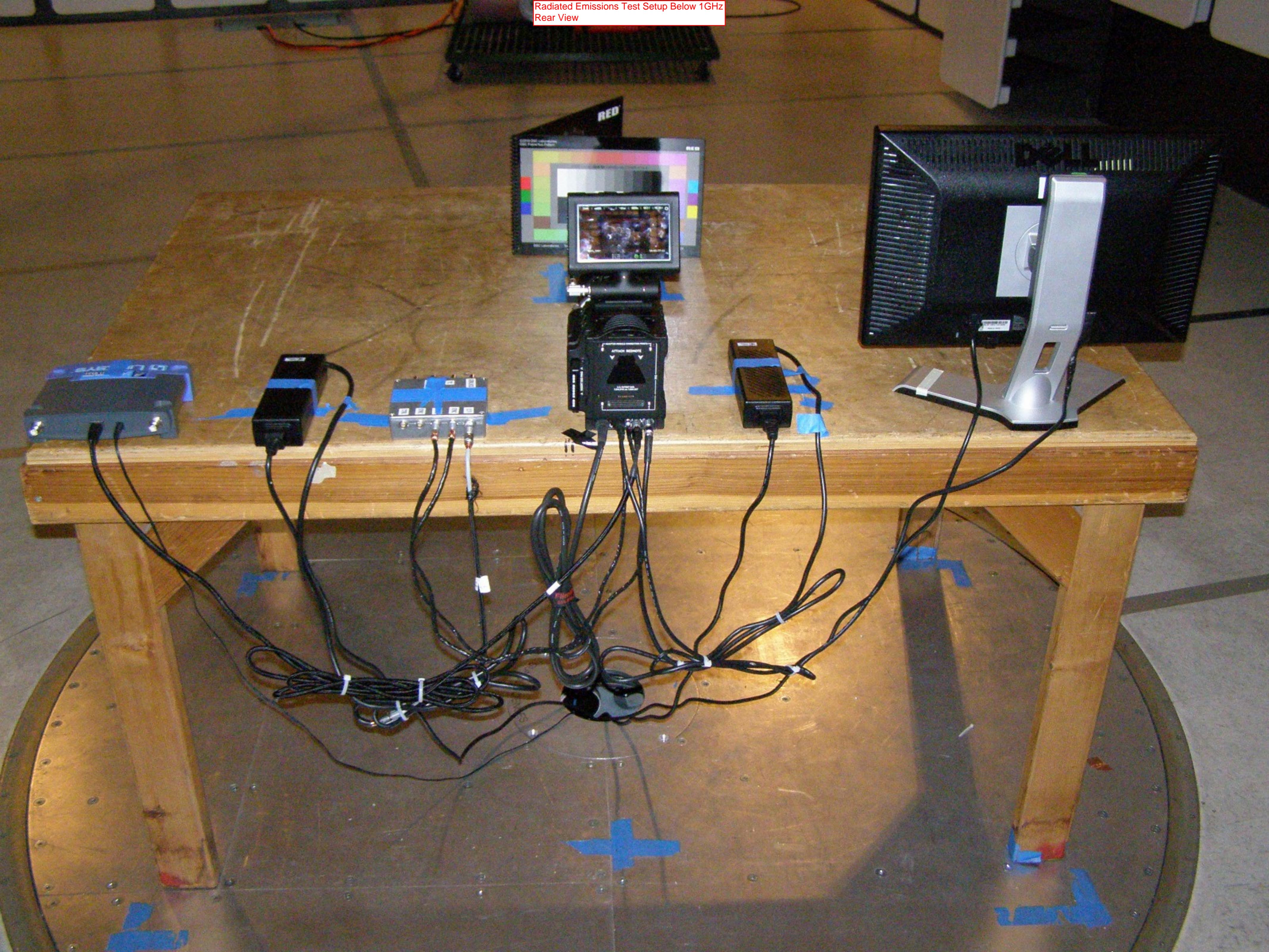
Radiated Emissions Test Setup Above 1GHz
