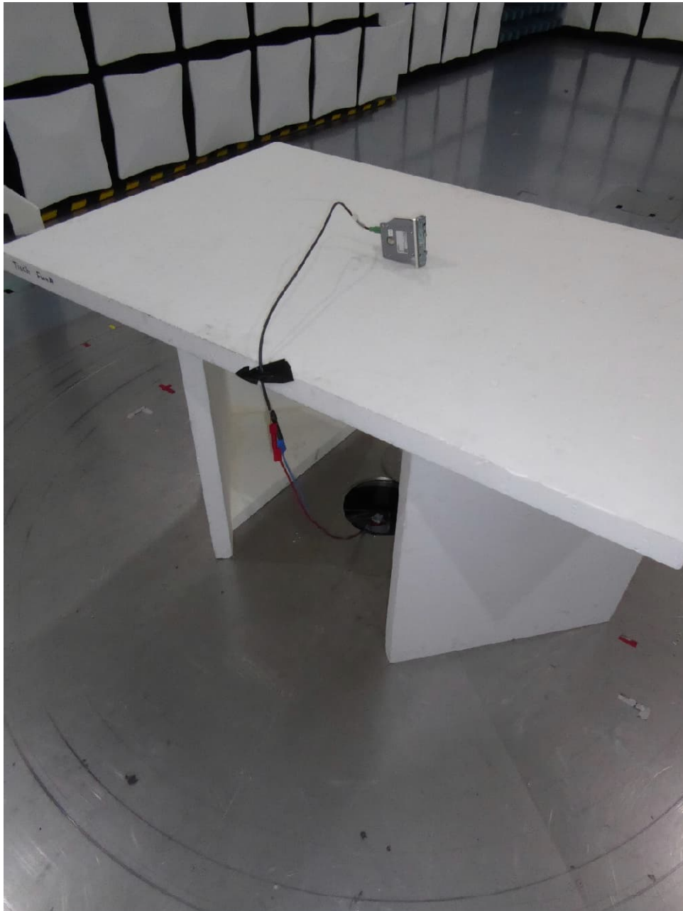
Test setup semi anechoic chamber (position 2)
