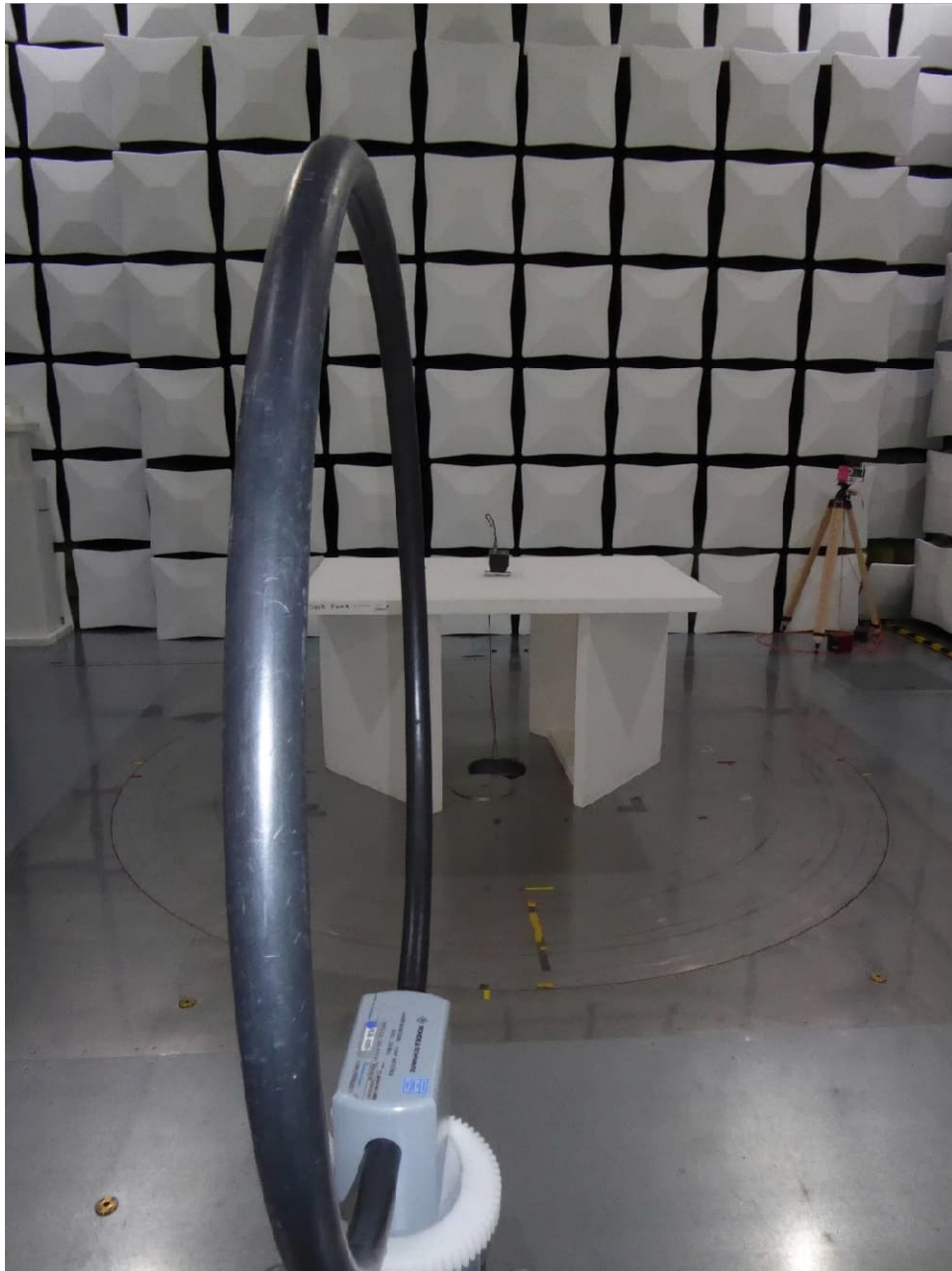
Test setup semi anechoic chamber <30 MHz
