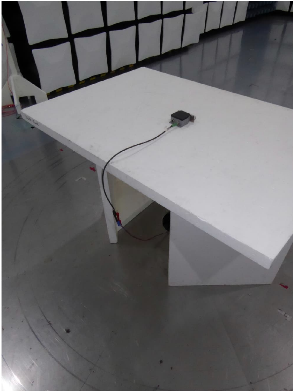
Test setup semi anechoic chamber (position 3)
