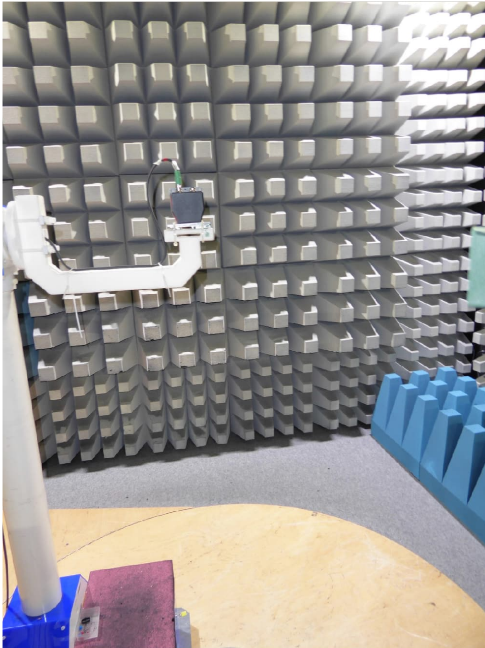
Test setup fully anechoic chamber <40 GHz
