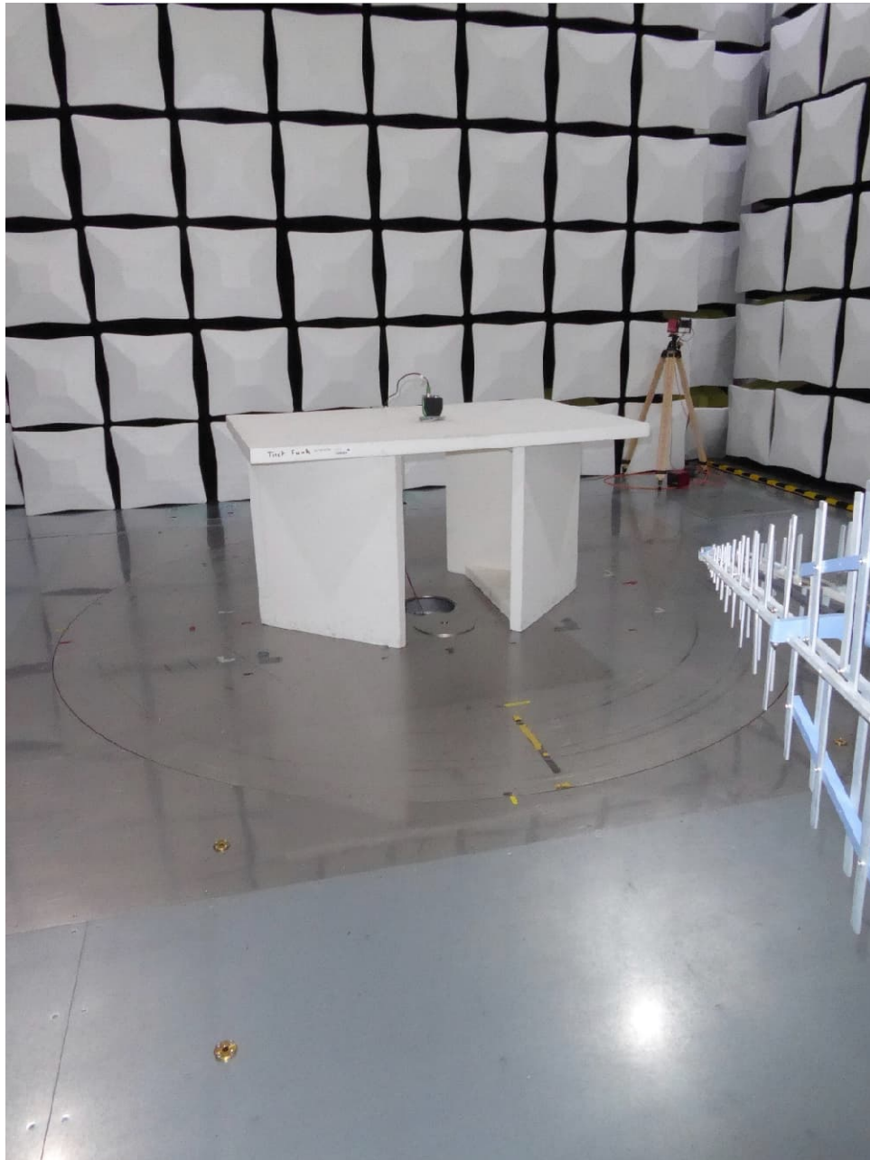
Test setup semi anechoic chamber <1 GHz
