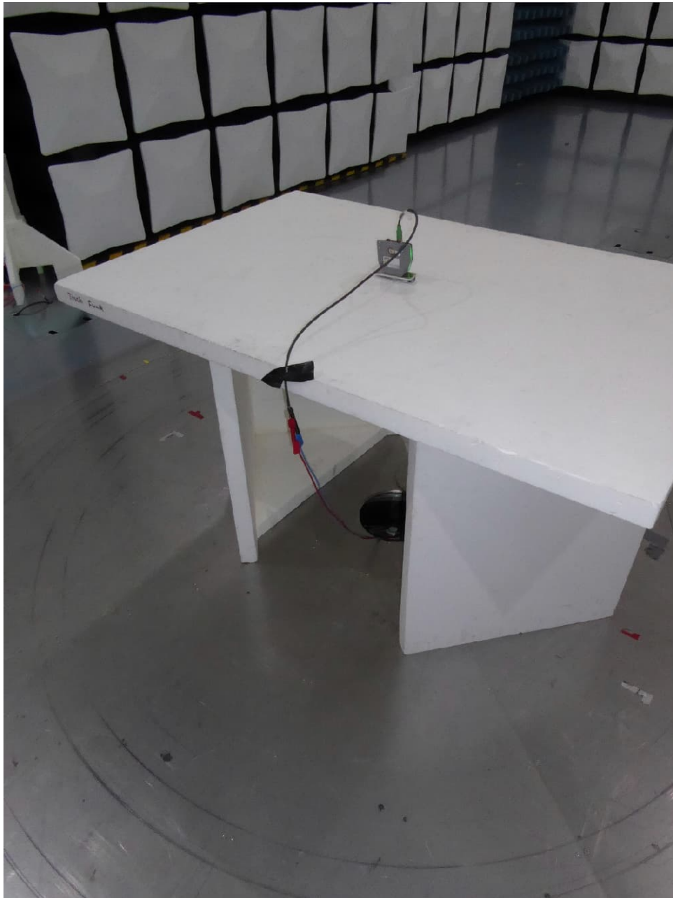
Test setup semi anechoic chamber (position 1)
