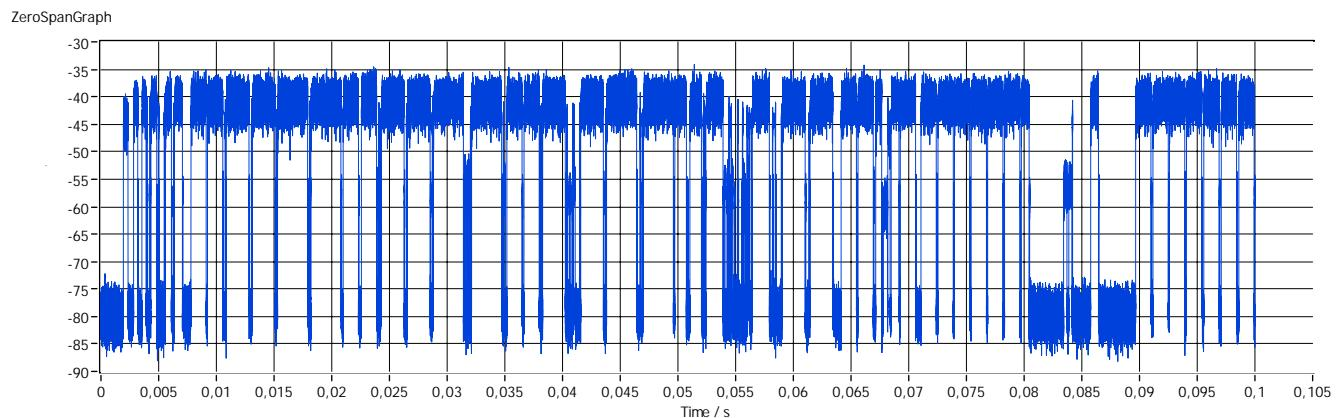
$$\text{Channel load} = \frac{\text{Time on}}{(\text{Time on} + \text{Off Time})} = \frac{26.64 \text{ ms}}{100 \text{ ms}} = 0.2664 \xrightarrow{\text{yields}} 26.6 \%$$
