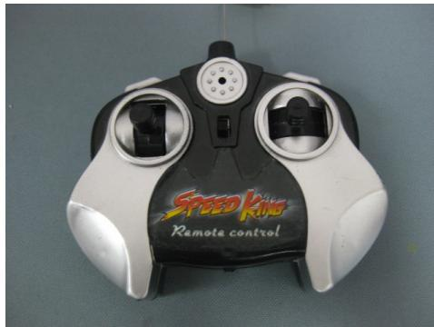
1. Unscrew the battery cover on the underside of the handset controller with a screwdriver.
