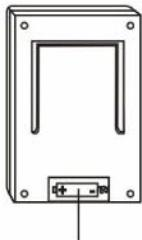
Insert batteries in the back of the light and remote as shown.
