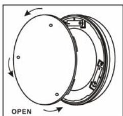
Twist the back cover of the light counter clockwise to open.
