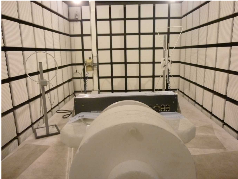
Photo 3: EUT at the anechoic chamber
