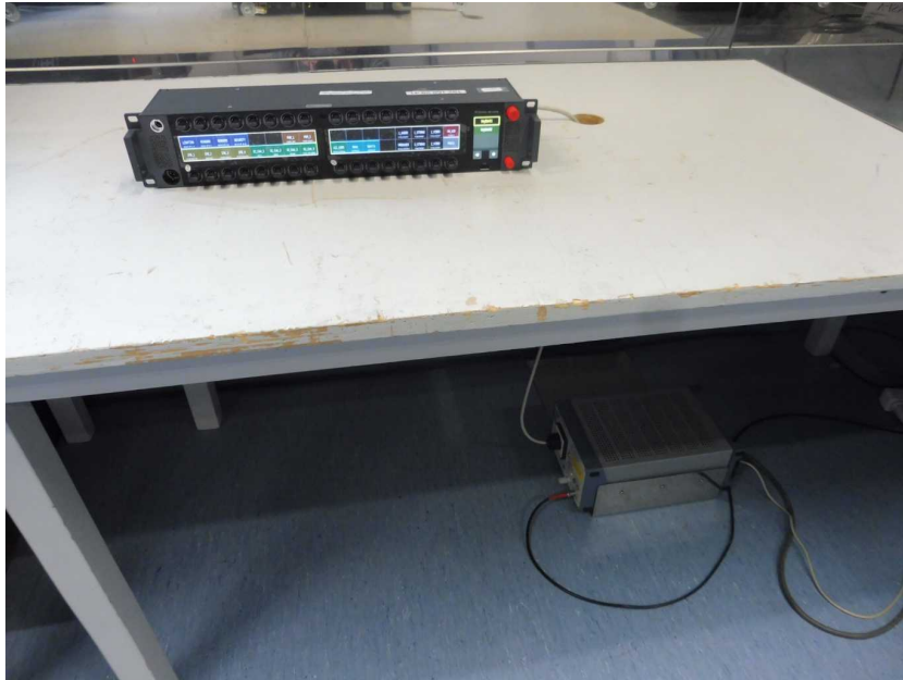
Photo 15: AC conducted emission test setup
