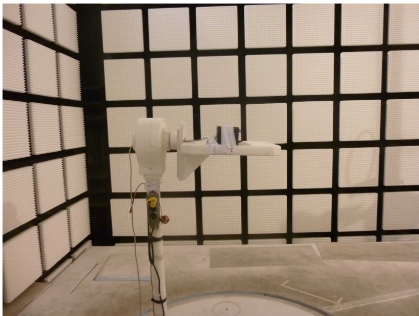
Photo 4: EUT at the anechoic chamber
