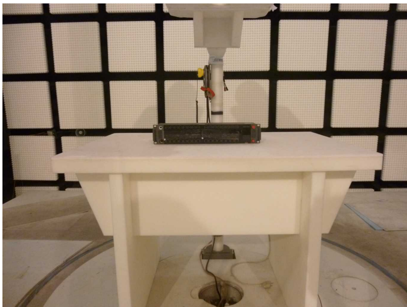
Photo 12: EUT at the anechoic chamber, loop antenna test setup
