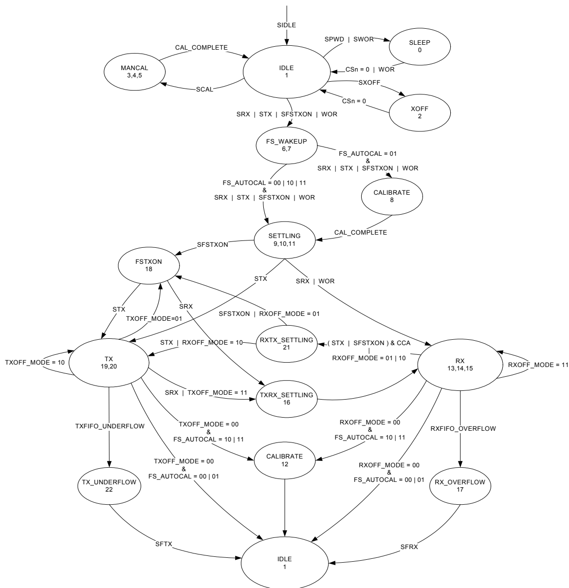
Figure 21: Complete Radio Control State Diagram
