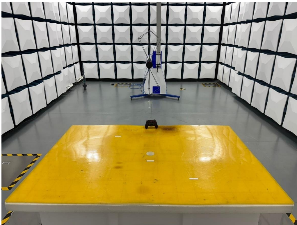
Set-up for Radiated Emission (30MHz-200MHz)
