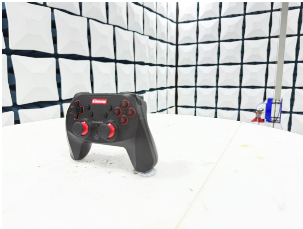
Set-up for Radiated Emission (1GHz above)
