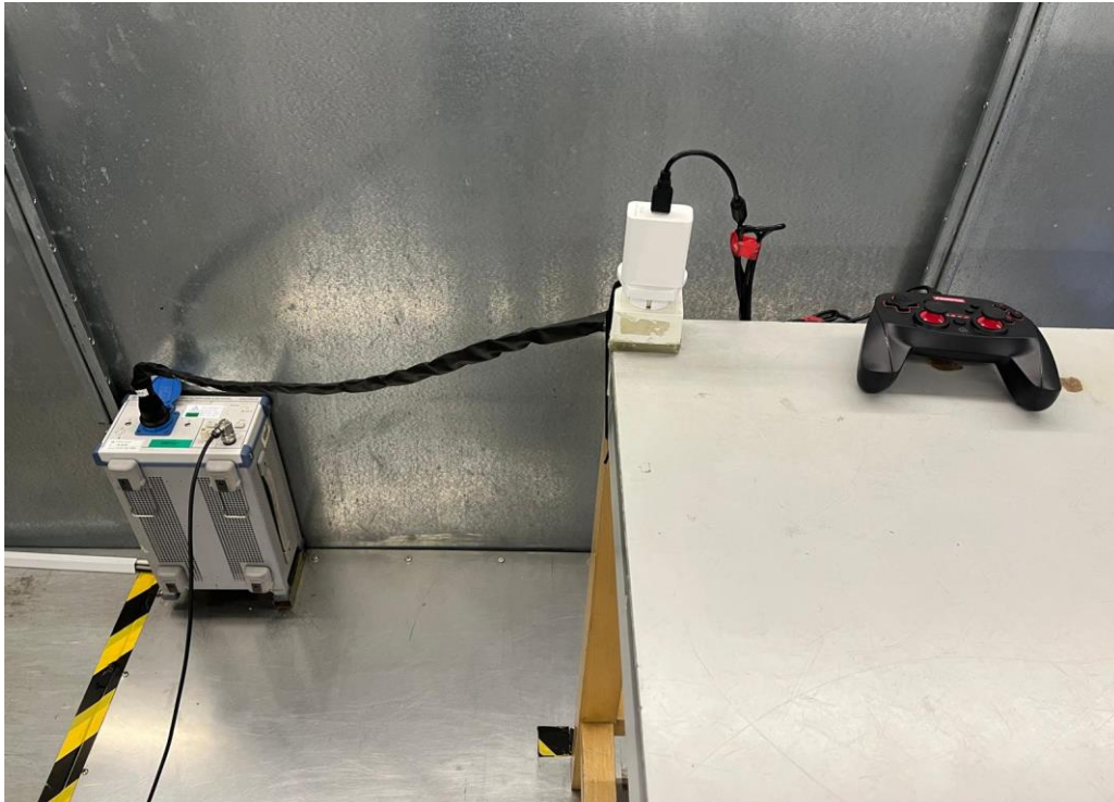
Set-up for Conducted Emission on AC Mains
