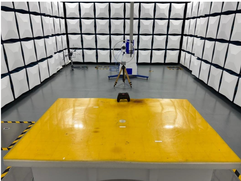
Set-up for Radiated Emission (9kHz-30MHz)
