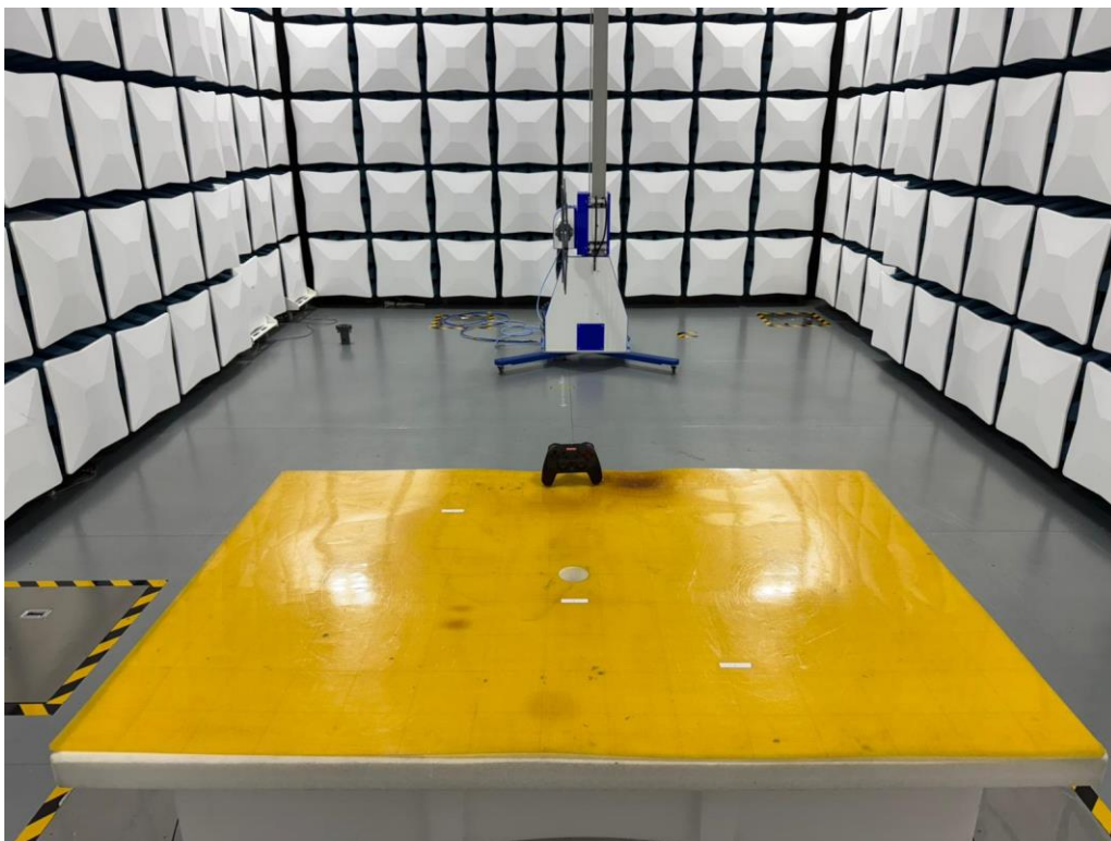
Set-up for Radiated Emission (200MHz-1000MHz)
