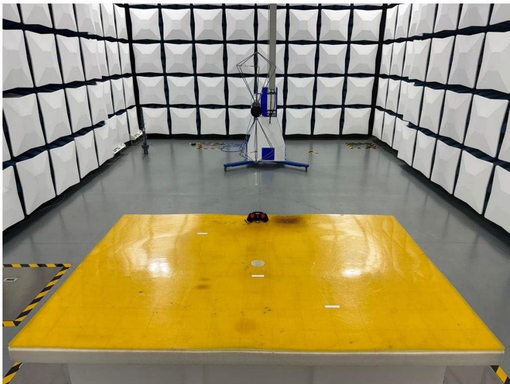
Set-up for Radiated Emission (30MHz-200MHz)
