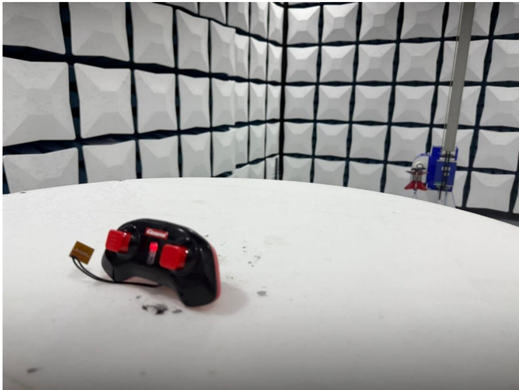
Set-up for Radiated Emission (1 GHz above)
