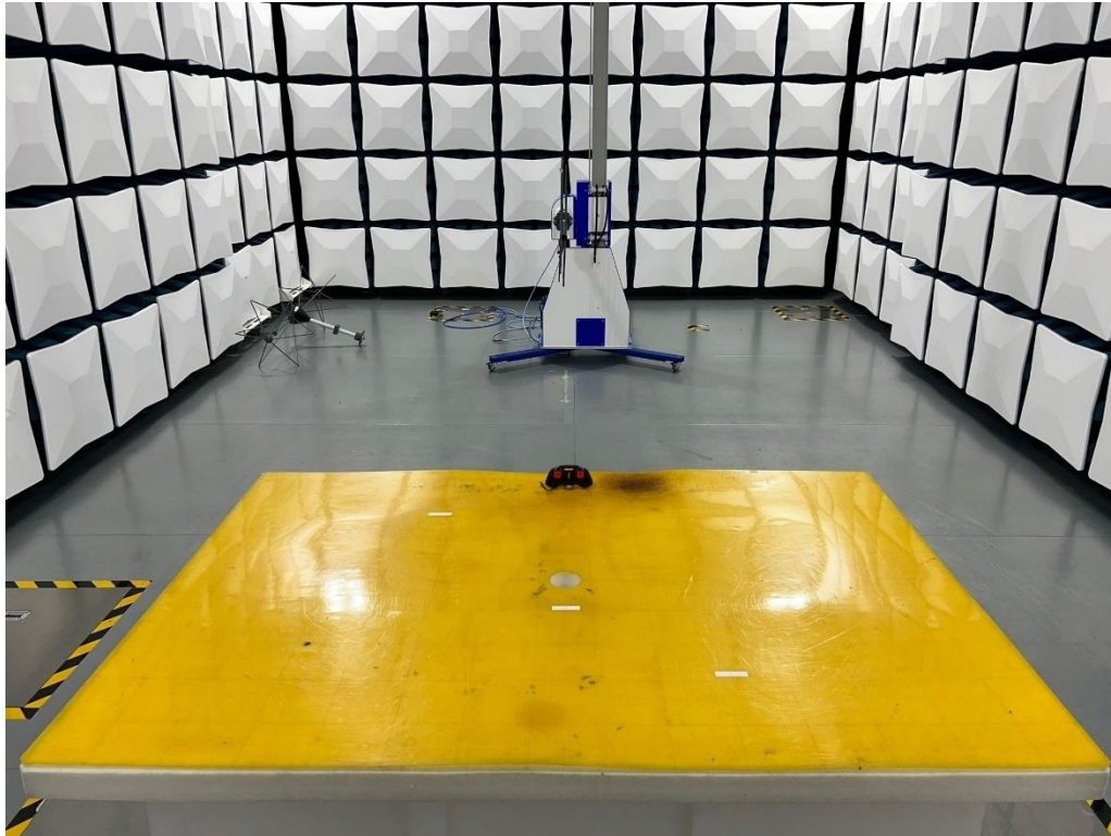
Set-up for Radiated Emission (200MHz-1000MHz)
