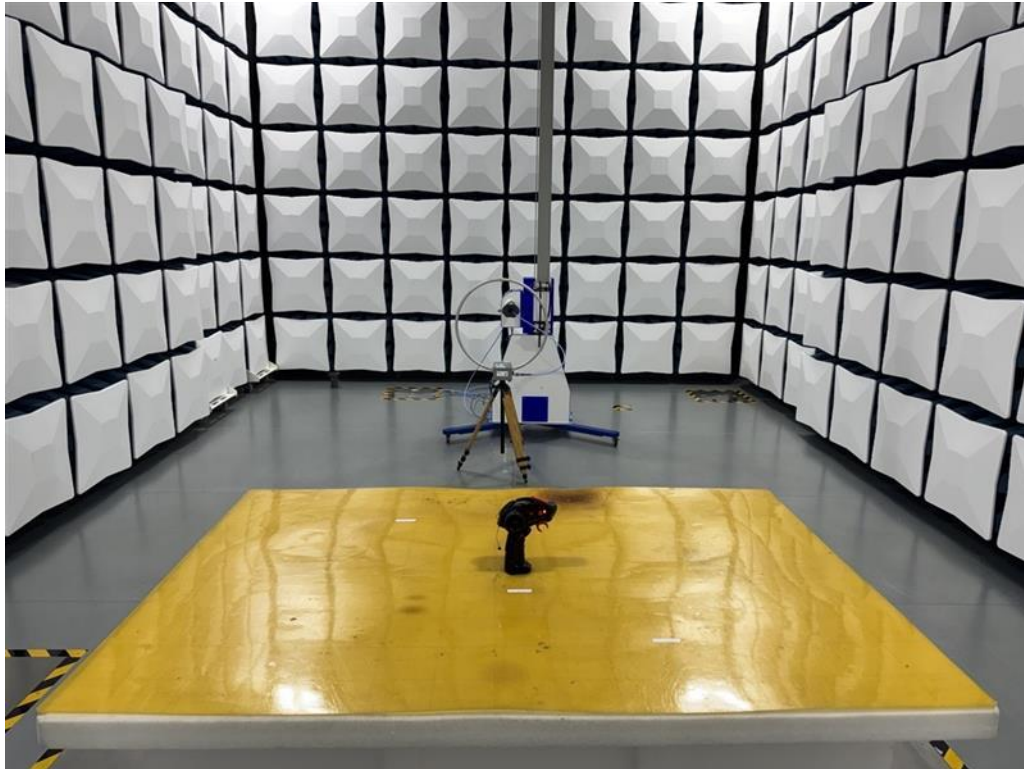
Set-up for Radiated Emission (9kHz-30MHz)
