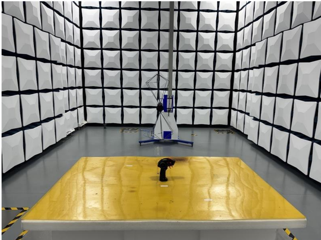
Set-up for Radiated Emission (30MHz-200MHz)
