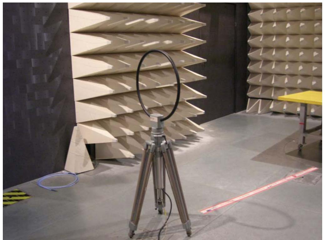
For radiated emissions 30MHz~1GHz
