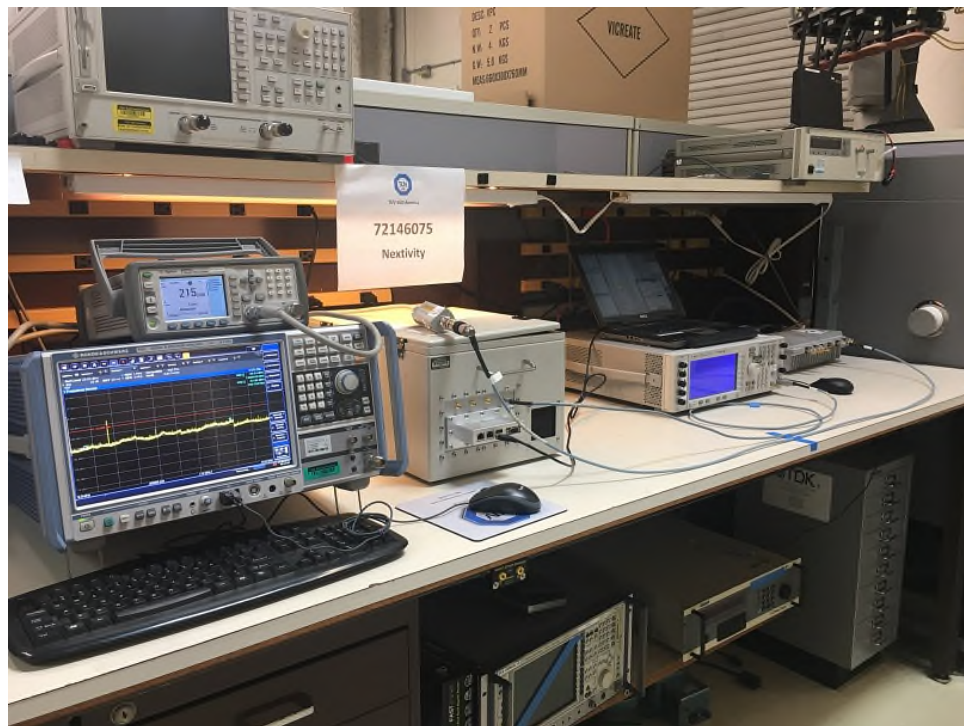
Conducted RF Testing
