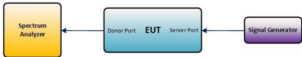
Figure 3 – Downlink test configuration in EUT test mode
