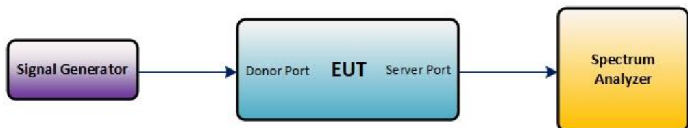
Figure 3 – Downlink test configuration in EUT test mode
