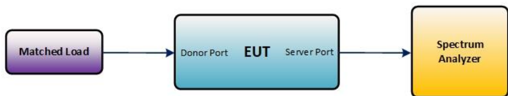
Figure 6 – Maximum downlink noise limit test configuration
