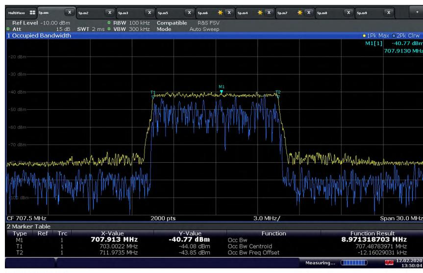
**LTE Band 12 Uplink (10 MHz BW) Mid Channel / 26 dB BW at Output port with Input signal at AGC + 3 dB Level**
