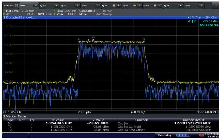
**LTE Band 2 Downlink (20 MHz BW) Mid Channel / 26 dB BW at Output port with Input signal at AGC + 3 dB Level**
