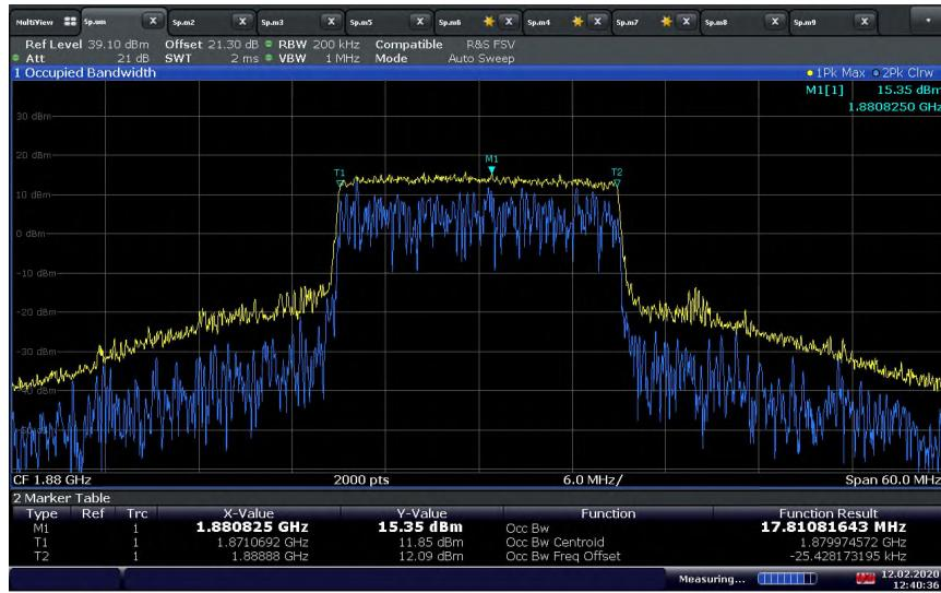
**LTE Band 2 Uplink (20 MHz BW) Mid Channel / 99% OBW at Input port (Adjusted Level)**
