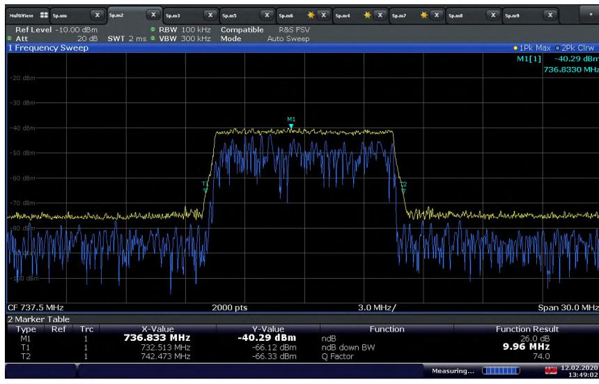
**LTE Band 12 Uplink (10 MHz BW) Mid Channel / 99% OBW at Output port with Input signal at AGC Threshold Level**
