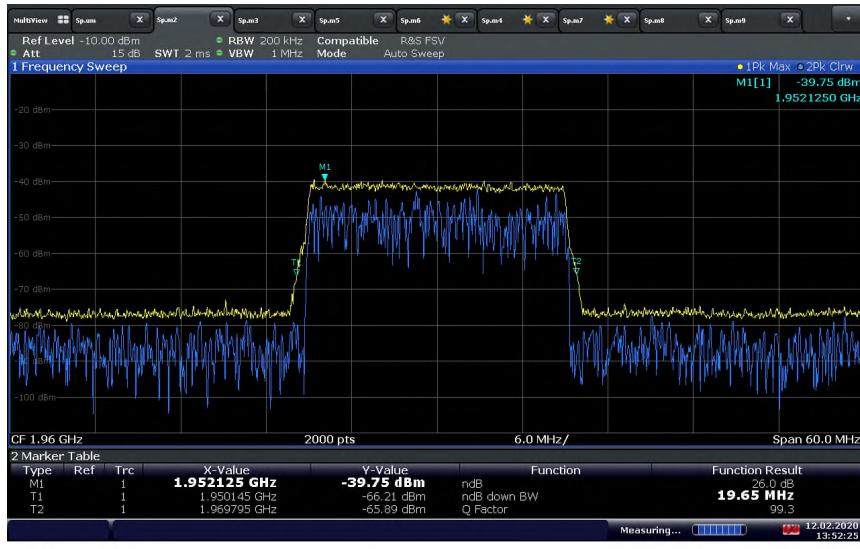
**LTE Band 2 Downlink (20 MHz BW) Mid Channel / 99% OBW at Output port with Input signal at AGC + 3 dB Level**
