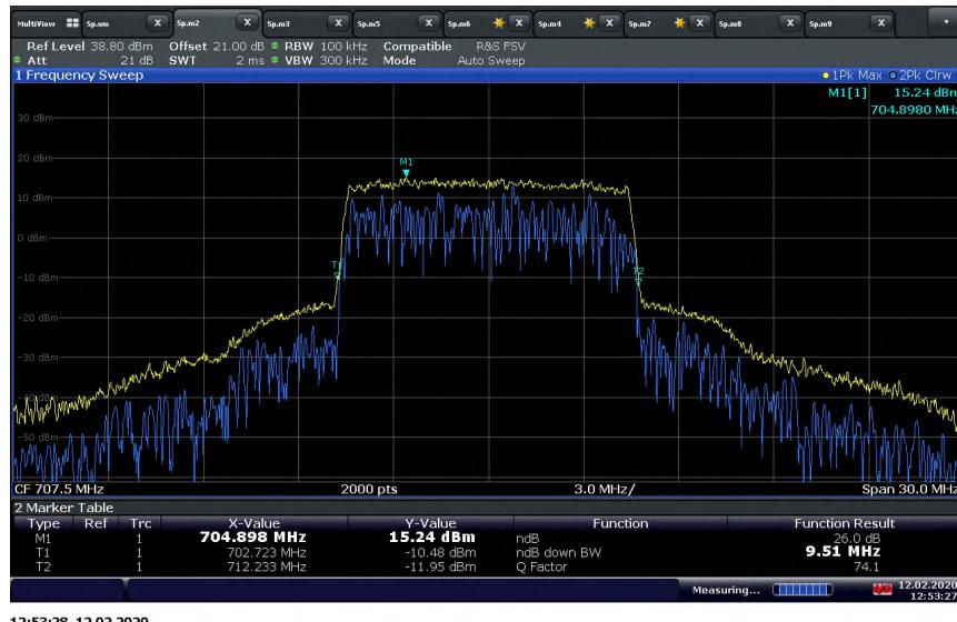
**LTE Band 12 Uplink (10 MHz BW) Mid Channel / 26 dB BW at Input port (Adjusted Level)**
