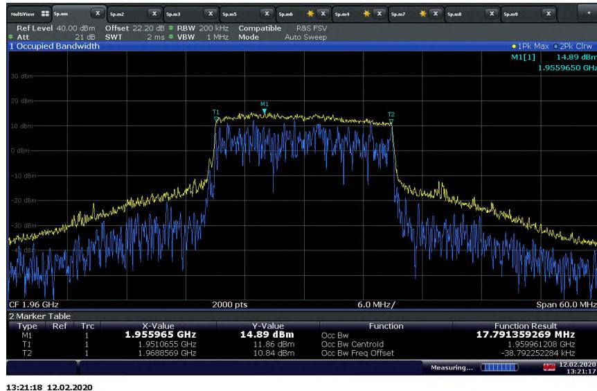
**LTE Band 2 Downlink (20 MHz BW) Mid Channel / 99% OBW at Input port (Adjusted Level)**
