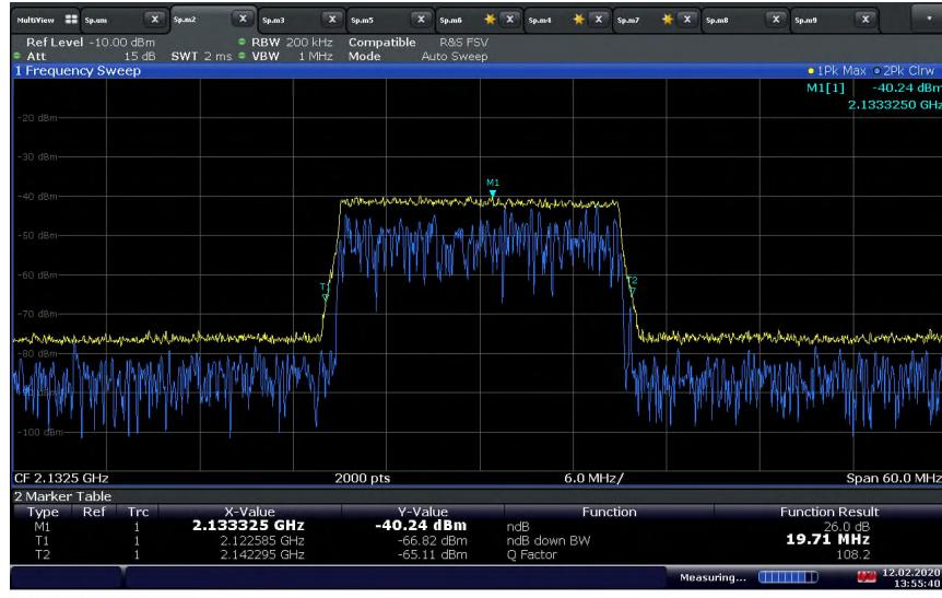
**LTE Band 4 Downlink (20 MHz BW) Mid Channel / 99% OBW at Output port with Input signal at AGC + 3 dB Level**
