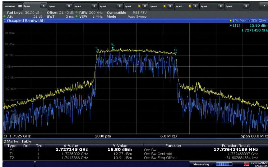
**LTE Band 4 Uplink (20 MHz BW) Mid Channel / 99% OBW at Input port (Adjusted Level)**
