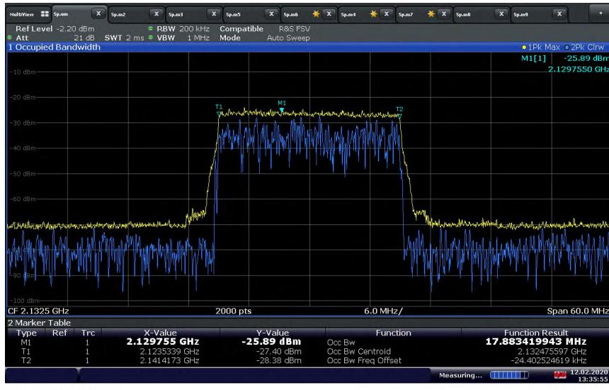
**LTE Band 4 Downlink (20 MHz BW) Mid Channel / 26 dB BW at Output port with Input signal at AGC + 3 dB Level**
