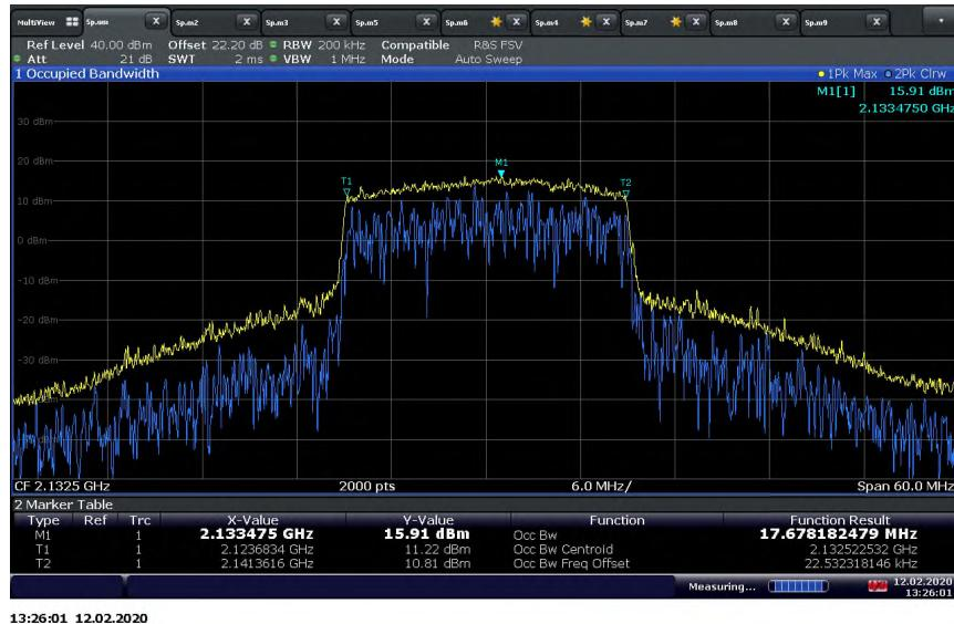
**LTE Band 4 Downlink (20 MHz BW) Mid Channel / 99% OBW at Input port (Adjusted Level)**
