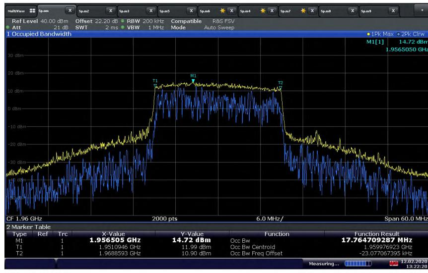
**LTE Band 2 Downlink (20 MHz BW) Mid Channel / 99% OBW at Input port (Adjusted Level)**
