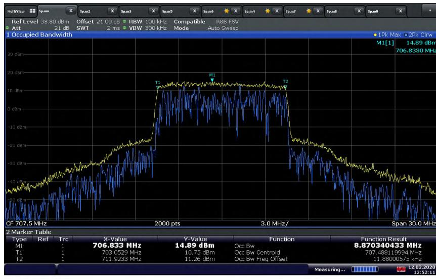
**LTE Band 12 Uplink (10 MHz BW) Mid Channel / 99% OBW at Input port (Adjusted Level)**
