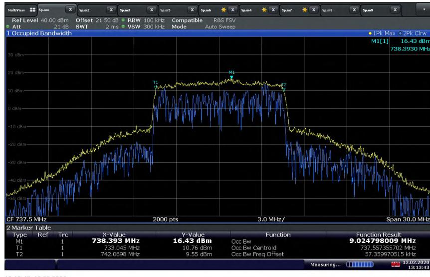
**LTE Band 12 Downlink (10 MHz BW) Mid Channel / 99% OBW at Input port (Adjusted Level)**
