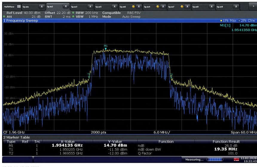
**LTE Band 2 Downlink (20 MHz BW) Mid Channel / 26 dB BW at Input port (Adjusted Level)**
