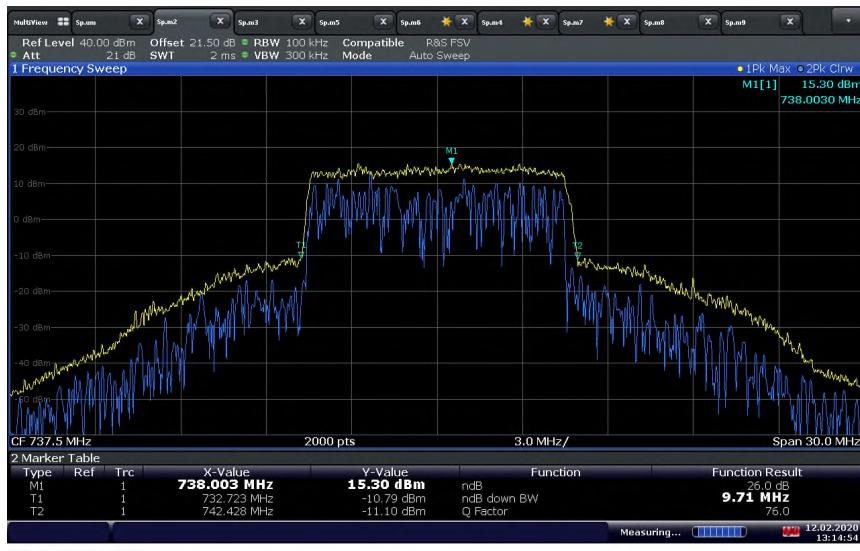
**LTE Band 12 Downlink (10 MHz BW) Mid Channel / 26 dB BW at Input port (Adjusted Level)**
