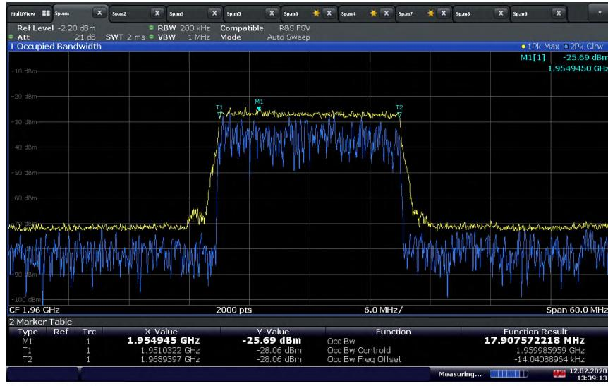
**LTE Band 2 Downlink (20 MHz BW) Mid Channel / 26 dB BW at Output port with Input signal at AGC Threshold Level**
