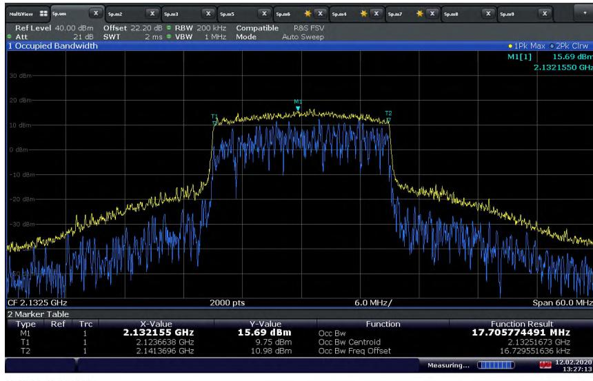
**LTE Band 4 Downlink (20 MHz BW) Mid Channel / 99% OBW at Input port (Adjusted Level)**
