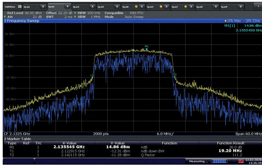
**LTE Band 4 Downlink (20 MHz BW) Mid Channel / 26 dB BW at Input port (Adjusted Level)**
