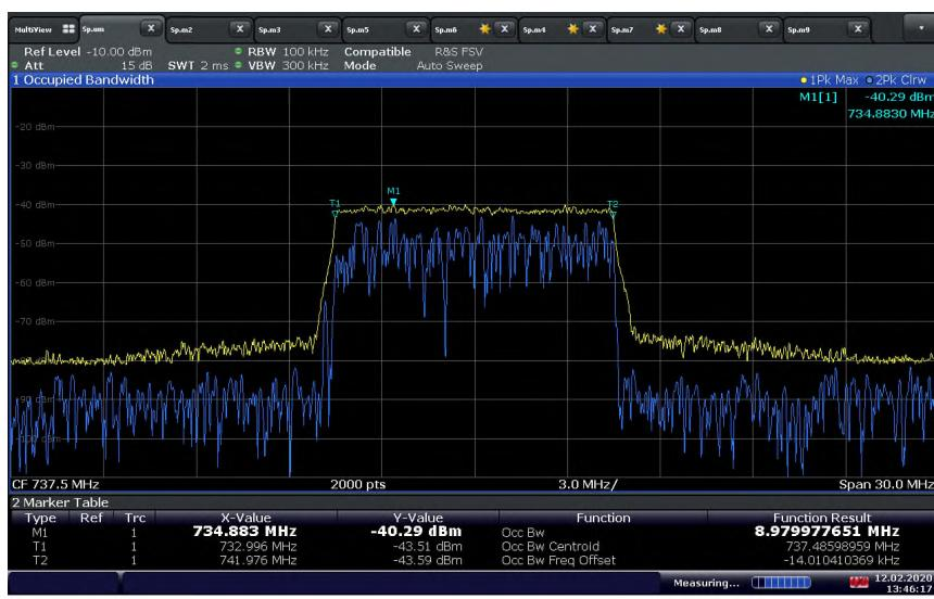
**LTE Band 12 Downlink (10 MHz BW) Mid Channel / 26 dB BW at Output port with Input signal at AGC + 3 dB Level**
