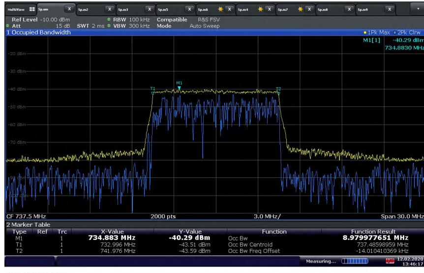
**LTE Band 12 Downlink (10 MHz BW) Mid Channel / 26 dB BW at Output port with Input signal at AGC Threshold Level**
