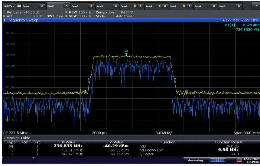
**LTE Band 12 Downlink (10 MHz BW) Mid Channel / 99% OBW at Output port with Input signal at AGC + 3 dB Level**
