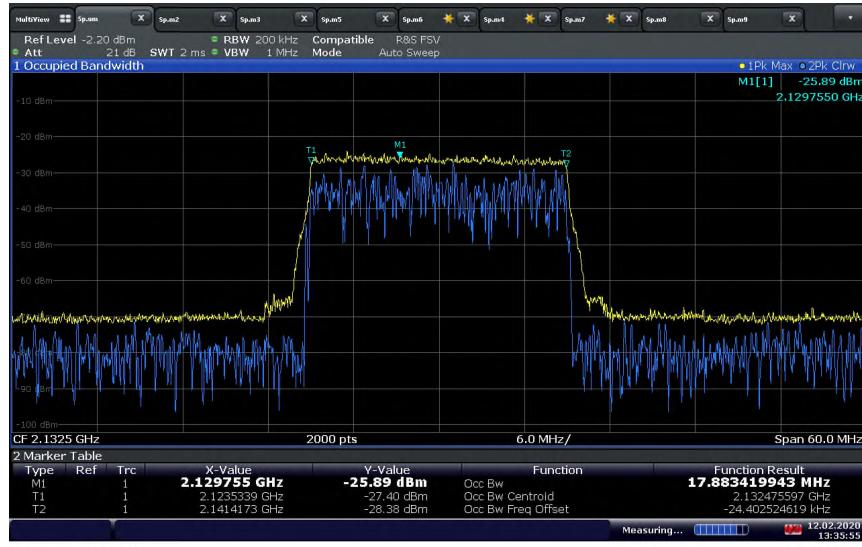
**LTE Band 4 Downlink (20 MHz BW) Mid Channel / 26 dB BW at Output port with Input signal at AGC Threshold Level**
