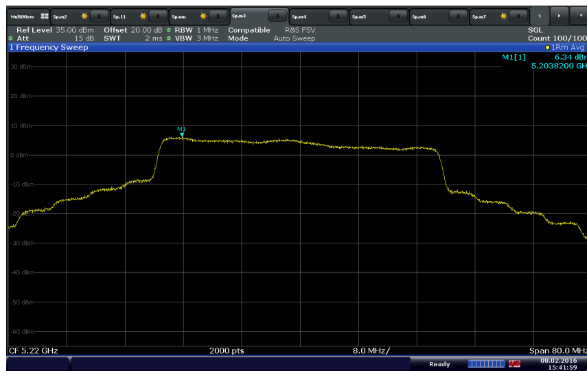
UNII 1 40MHz Bandwidth Mid Channel 5220 MHz
