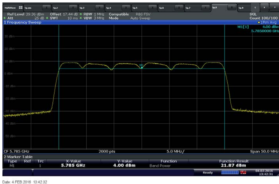
UNII 3 30MHz Bandwidth Middle Channel 5785 MHz
