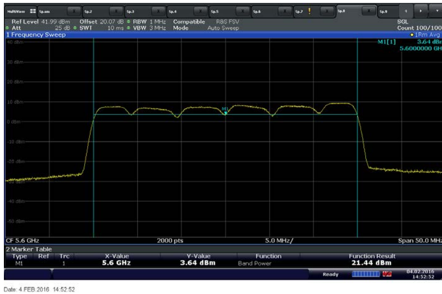
UNII 2C 30MHz Bandwidth Middle Channel 5600 MHz
