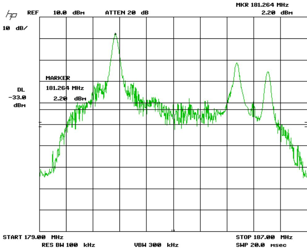
Note: For Band edge measurements, see spurious radiated emissions. There was 20 dB of external attenuation taken during this measurement.
