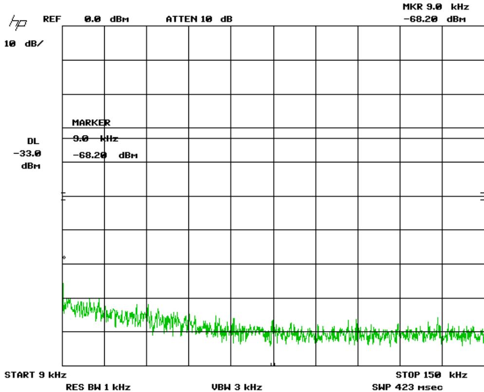
Note: Hi, middle and low were scanned, worst case antenna conducted is shown. There was 20 dB of external attenuation taken during this measurement.
