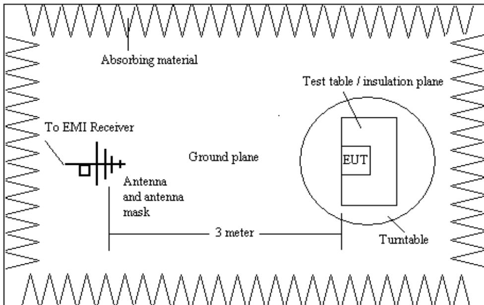
1. The pre-test of the radiated emissions test was conducted in a semi-anechoic chamber and the final measurement was conducted in the open area test site.
