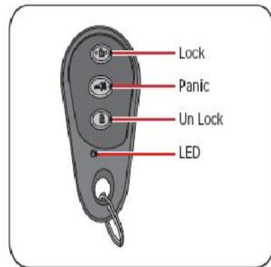
The front side of the RKE has control buttons and an LED. If the LED is not flashing when any of the buttons are pressed or when it flashes once when a button is pressed continuously, it indicates that the Remote Battery is low..
