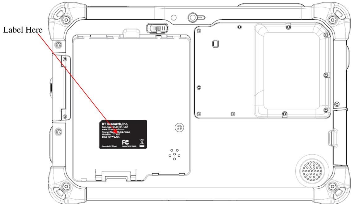
The label shown shall be permanently affixed at a conspicuous location on the device and be readily visible to the user at the time purchase (Labeling requirements per 2.925)
