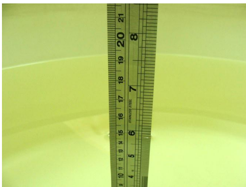
Fig 6.1 Photo of Liquid Height for Body SAR
