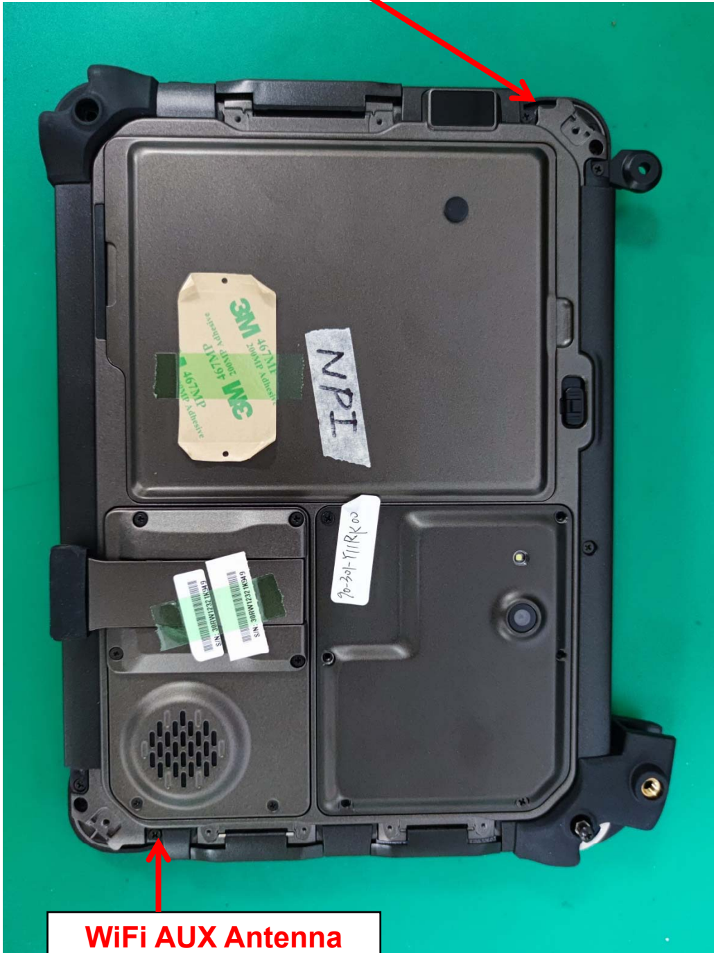
WiFi Main Antenna
