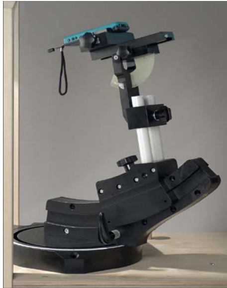
F-2. Device Holder for Transmitters
