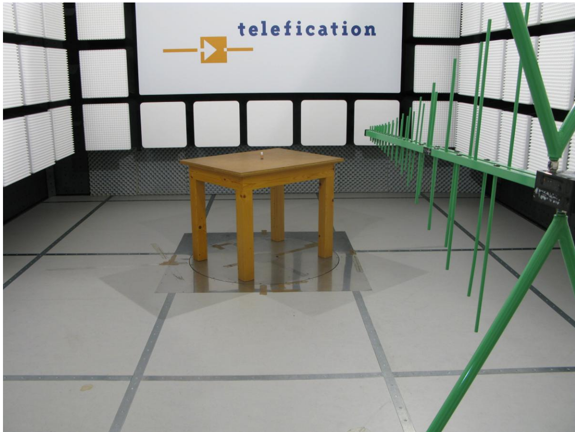
Photograph 1: - Test setup radiated emissions (30 - 1000 MHz)
