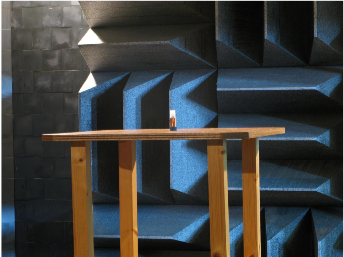
Photograph 4: - Test setup radiated emissions (1 - 5 GHz)
