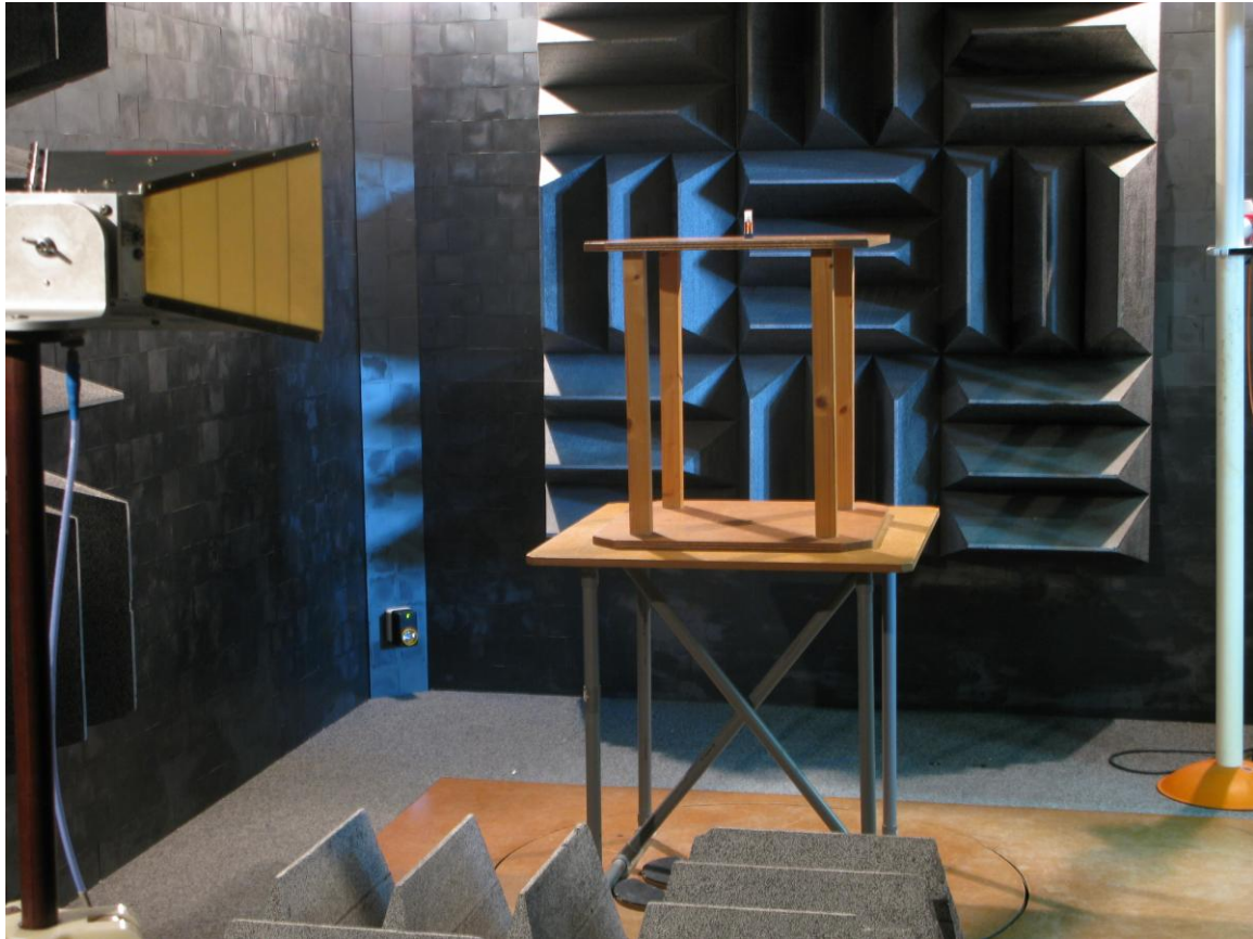
Photograph 3: - Test setup radiated emissions (1 - 5 GHz)
