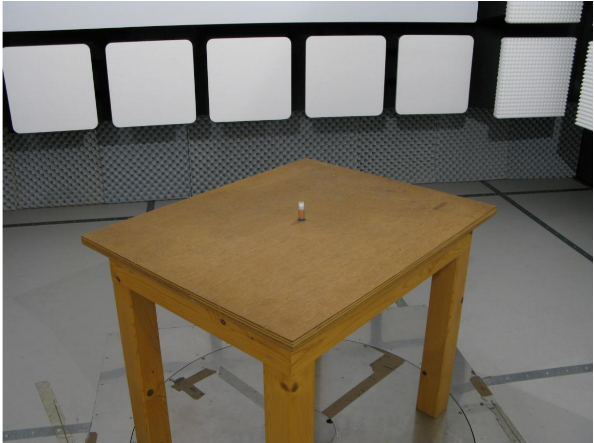
Photograph 2: - Test setup radiated emissions (30 - 1000 MHz)
