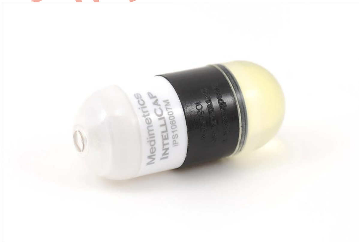
Figure 5: Photograph of an IntelliCap Capsule used for drug delivery and monitoring in a test subject.
