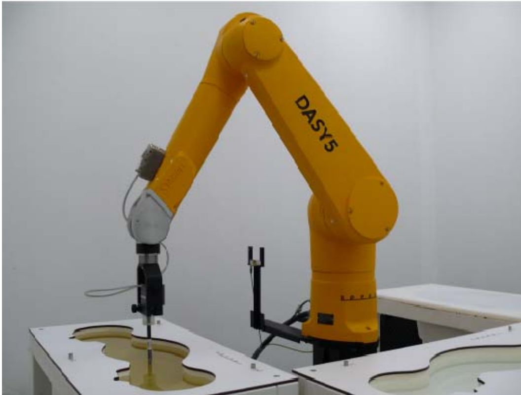
Picture 1: Specific Absorption Rate Test Layout
