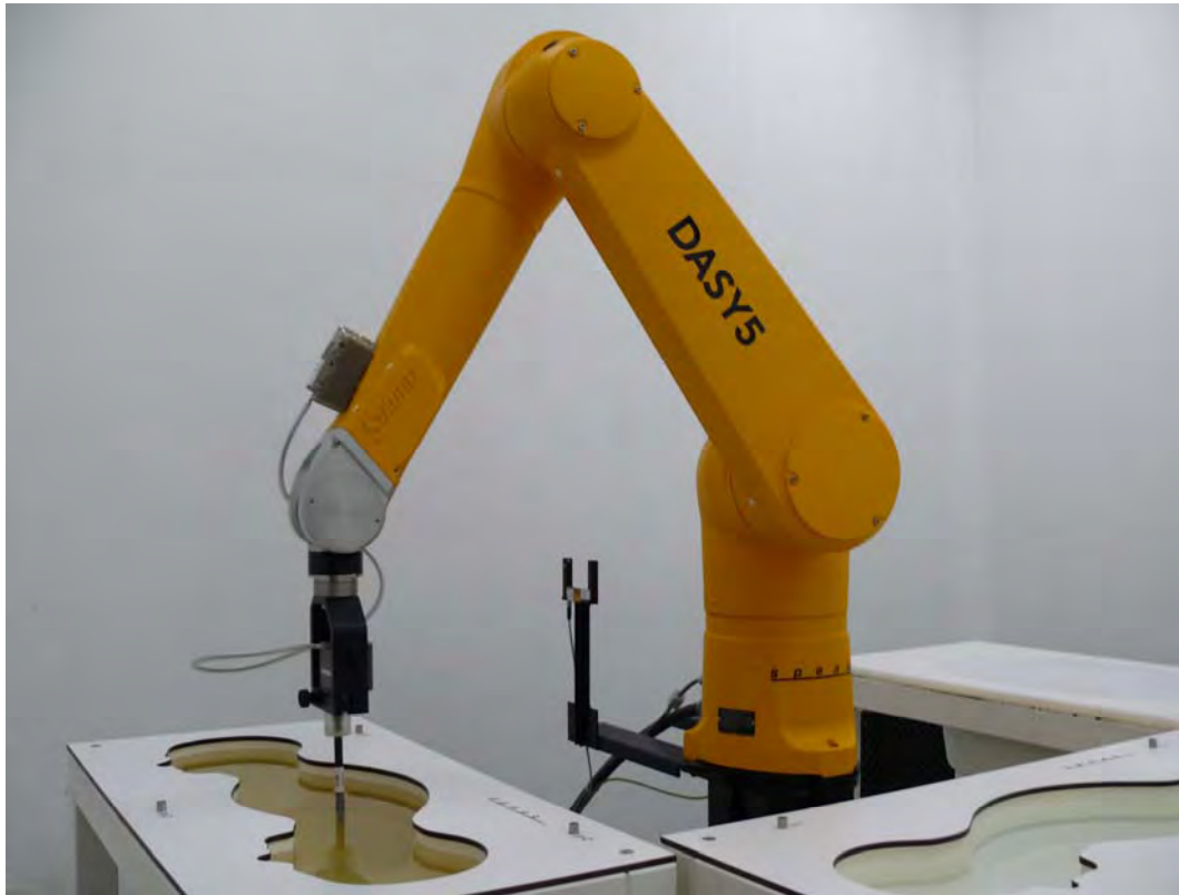
Picture 1: Specific Absorption Rate Test Layout
