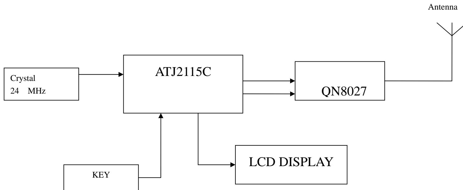
The power supply of CA001 is by DC 12V form adapter and it supply the power to ATJ2115C, ATJ2115C is the FM MCU module, It is connected with KEY part and LCD Display part, it send the FM signal via QN8027 to Antenna and transmitting.
