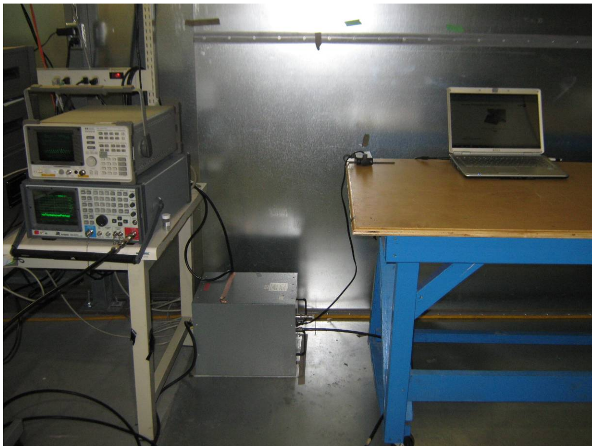
Power Line Conducted Emissions Test Setup
