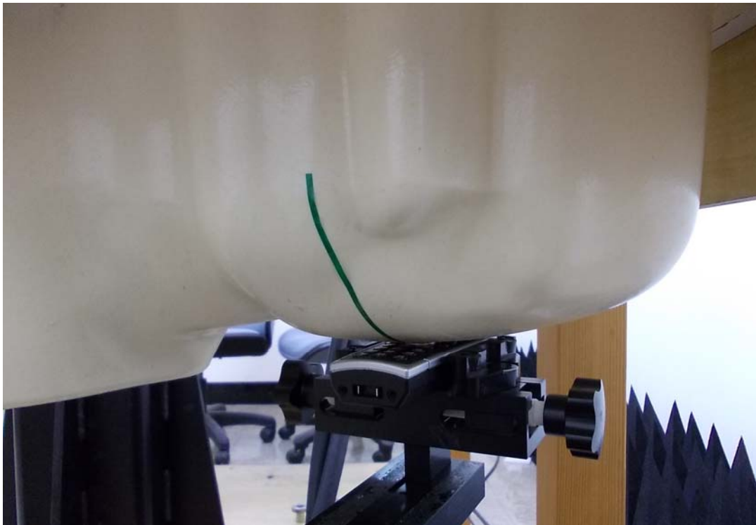
Measurement Position of Left-Cheek (LC) with Handset
