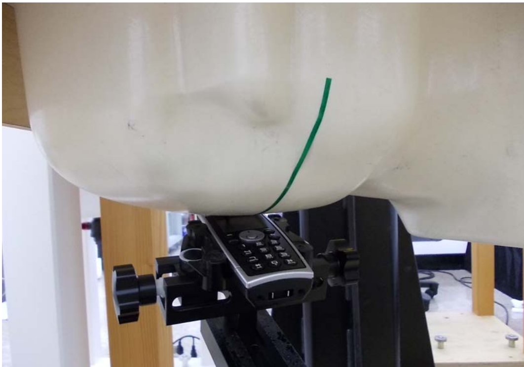
Measurement Position of Right-Tilt (RT) with Handset
