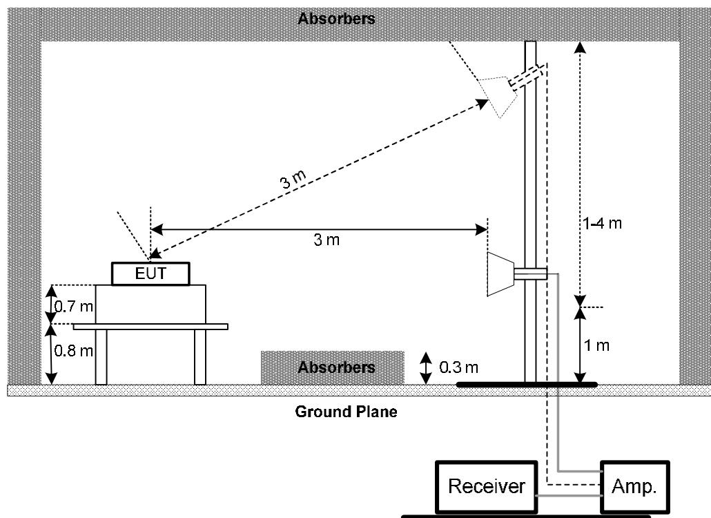
(C) For radiated emissions below 30MHz
