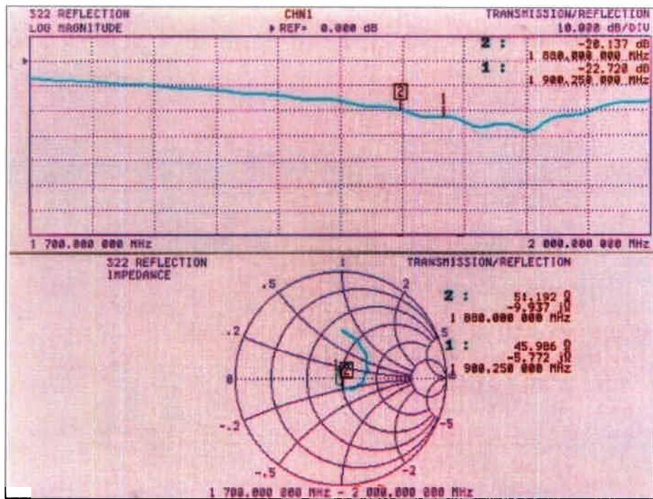
Dipole impedance at 1900 MHz  $\text{Re}\{Z\} = 46.0 \Omega$
