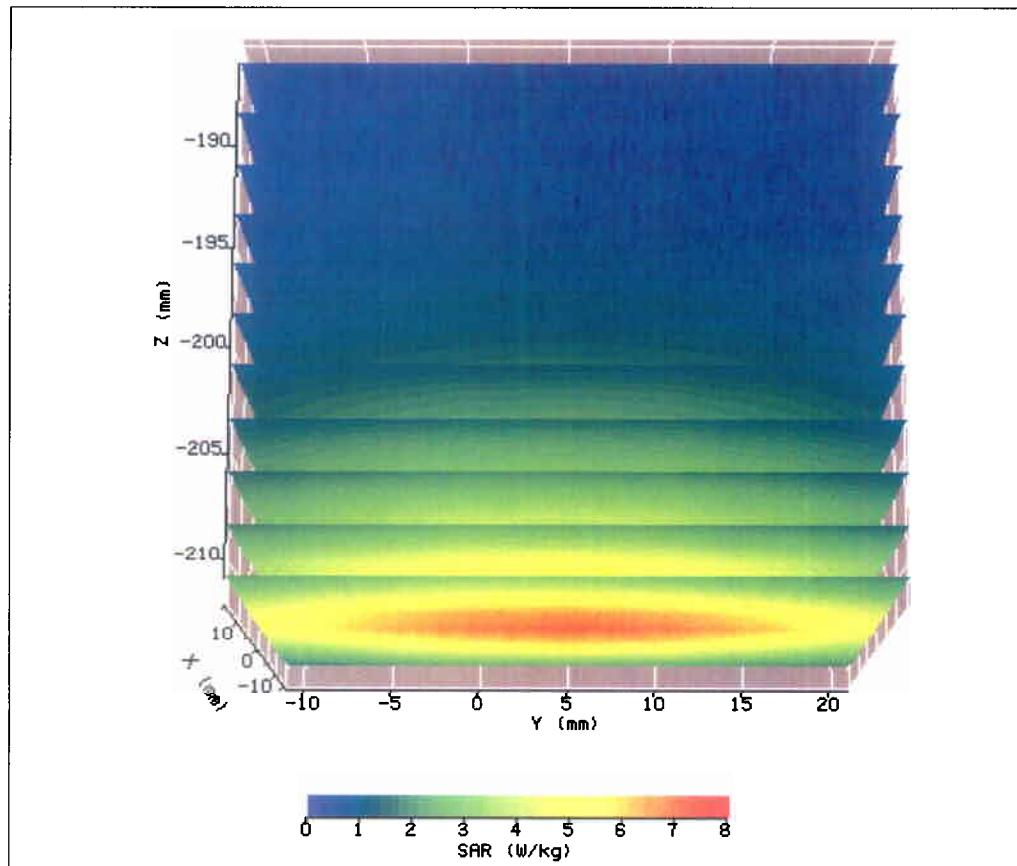
SAR measurement standard 62209-1 [ref 2] tabulates the volume-averaged 1g and 10g SAR values over a range of frequencies up to 3000MHz. The following values are listed for 1900MHz:
