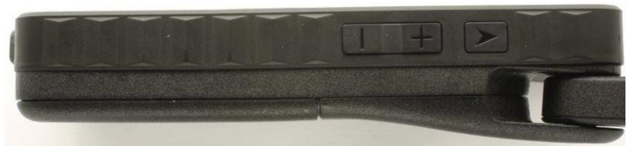
Side view, volume and tracking keys, antenna extended
