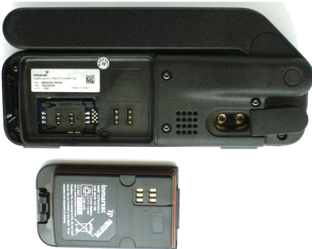
Back view, battery removed, back RF cover open
