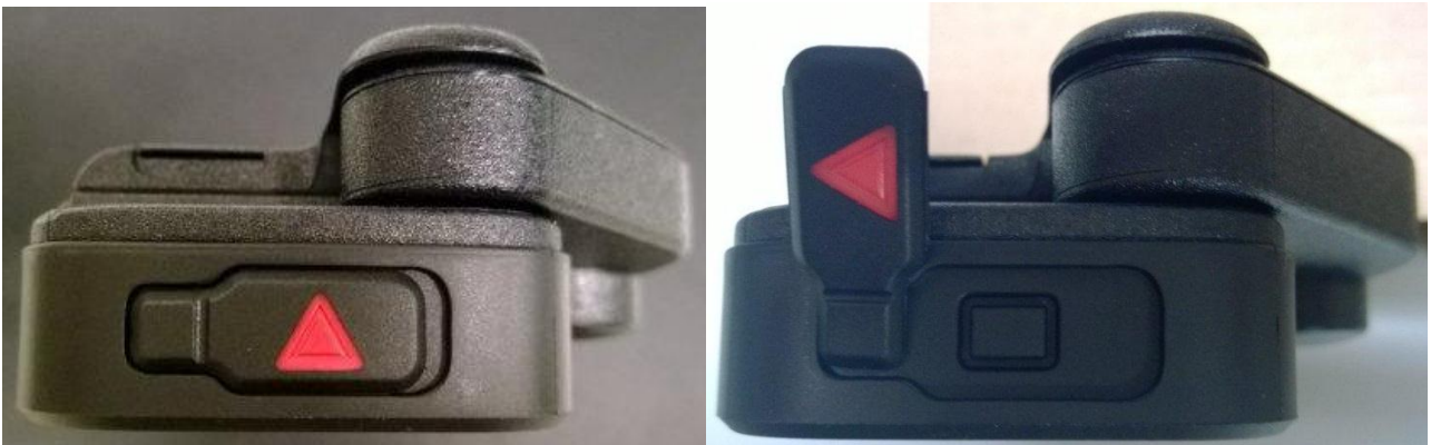
Bottom View, with audio and USD cover closed and in open position
