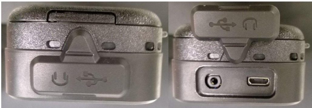
Bottom View, with audio and USD cover closed and in open position
