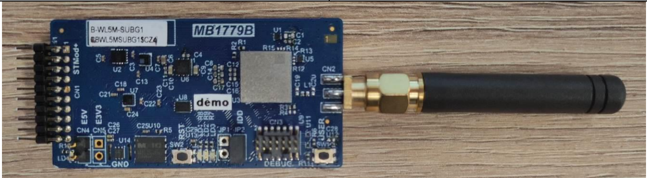
Test board (top side with module and antenna)
