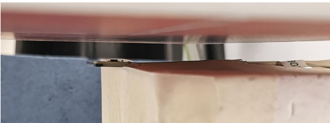
Figure 15 Back test position, RF Energy Enhancement, 10mm separation distance
