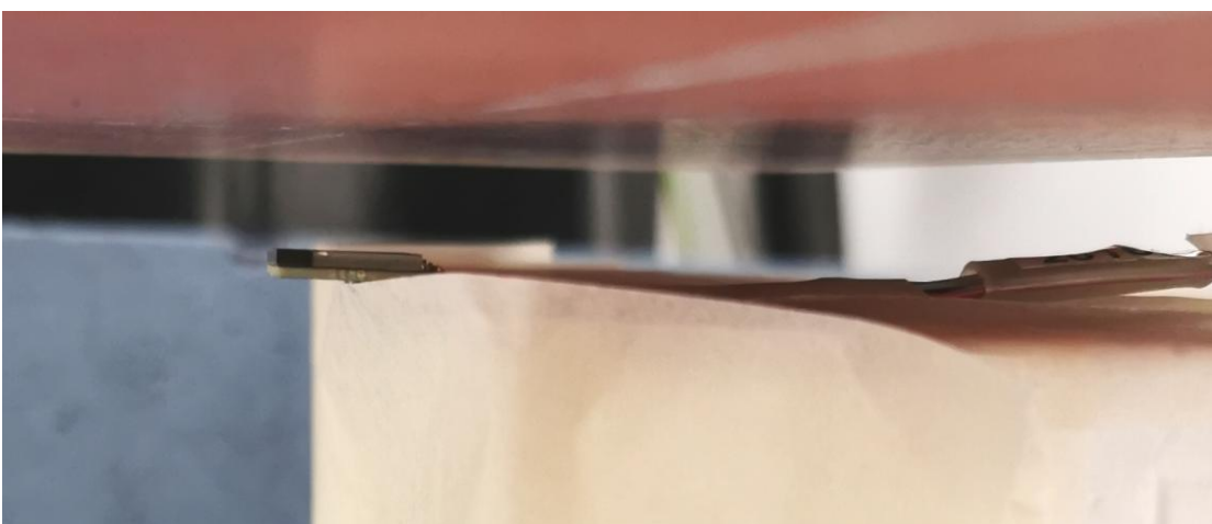
Figure 12 Front test position, RF Energy Coupling Enhancement, 10mm separation distance
