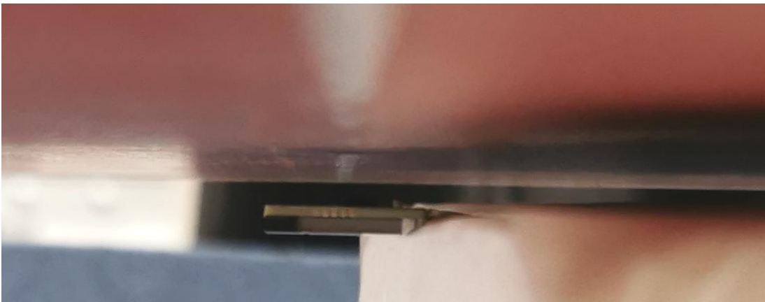
Figure 14 Back test position, RF Energy Enhancement, 5mm separation distance
