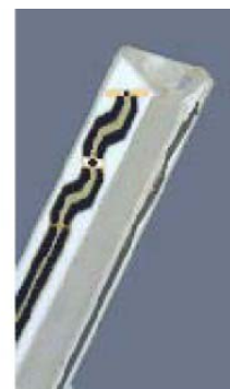
Figure 3.3 Probe Thick-Film Technique
