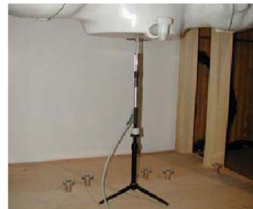
Figure 11.1 Dipole Verification Test Setup Diagram & Photo
