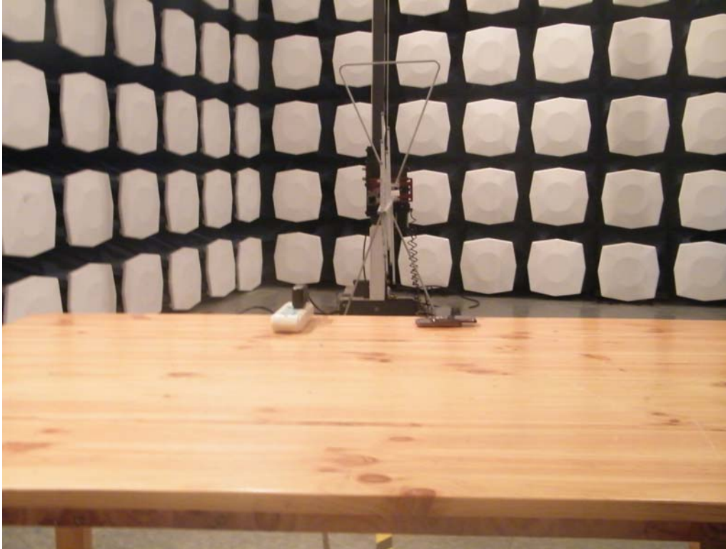
Picture 2 Radiated Emission Test Setup
