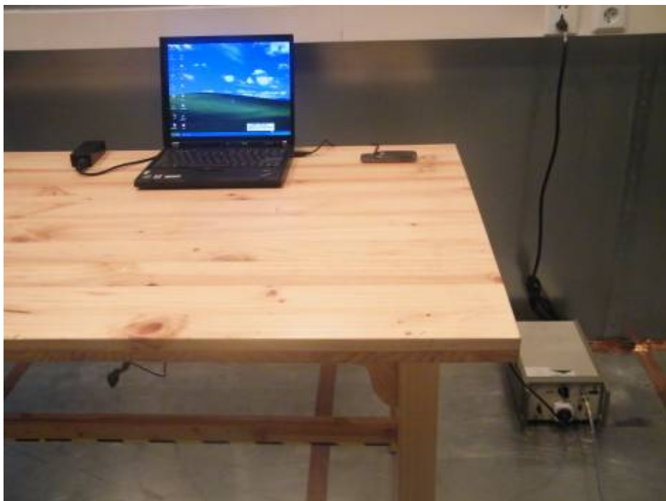
Picture 3 Conducted Emission Test Setup
