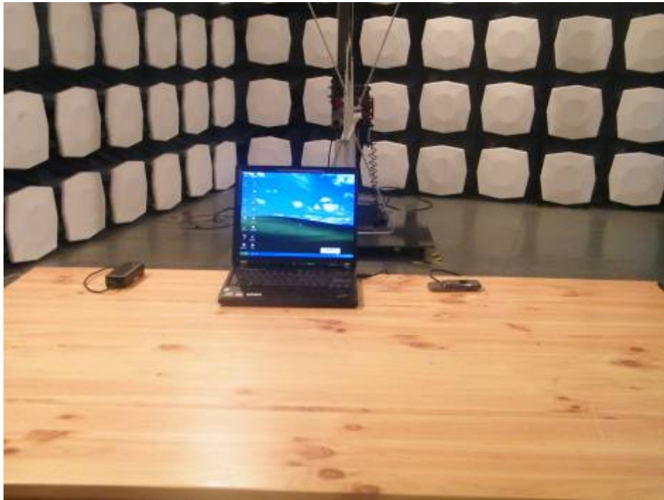
Picture 2 Radiated Emission Test Setup
